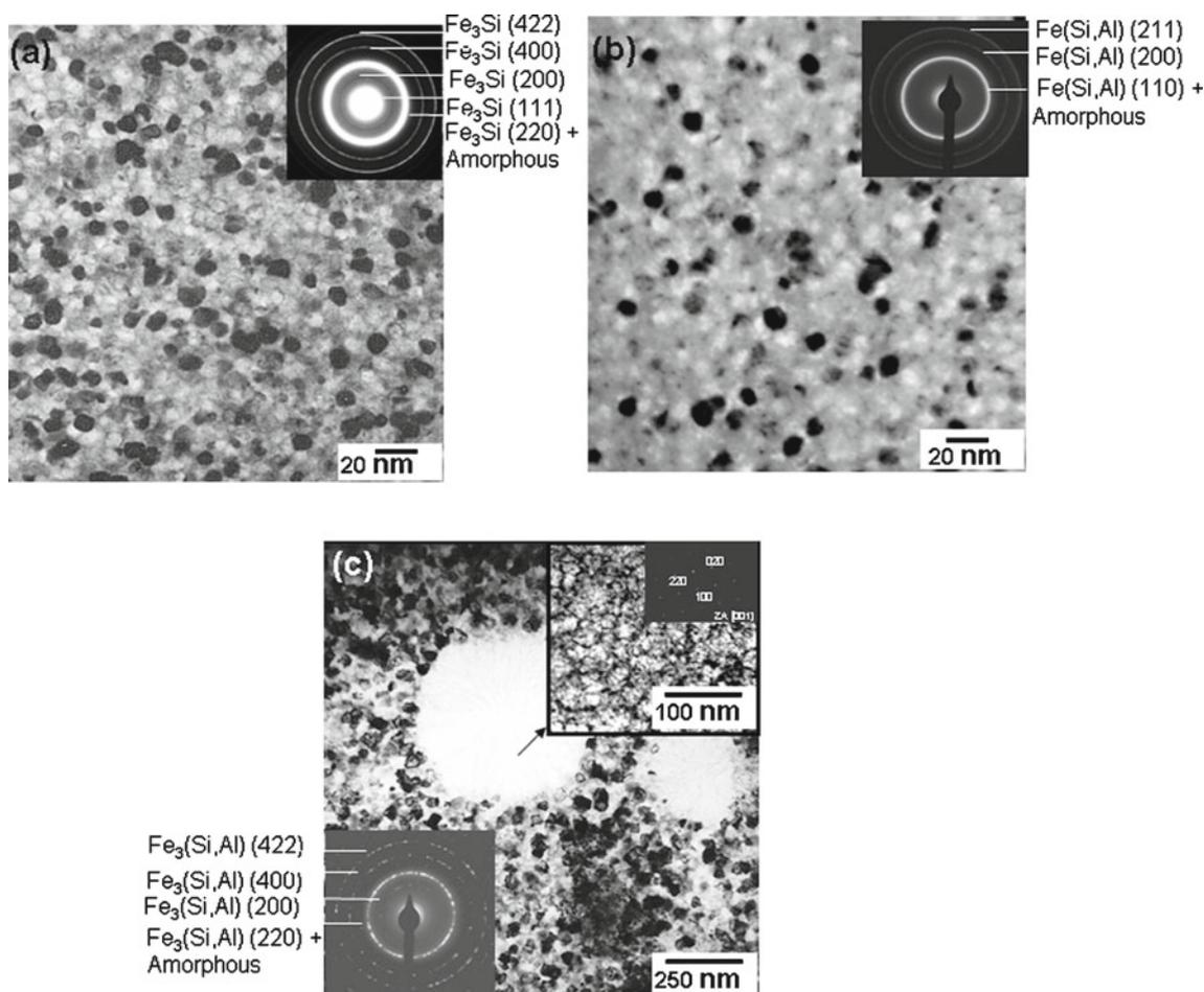
Figure 5. TEM images of (a) Al0, (b) Al2 and (c) Al6 annealed ribbons (insets: corresponding SAD patterns).
