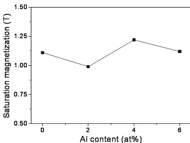
Figure 6. Saturation magnetization of annealed ribbons as a function of Al content.
