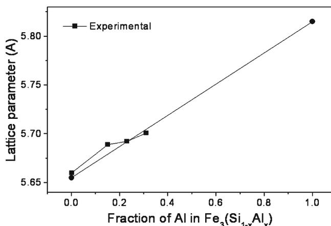
Figure 8. Variation of lattice parameter with Al content.
