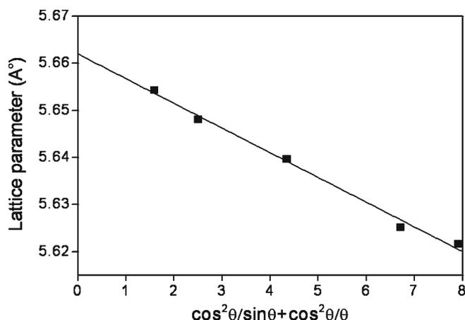
Figure 4. Lattice parameter as a function of *N-R* function for annealed Al0 ribbon.
