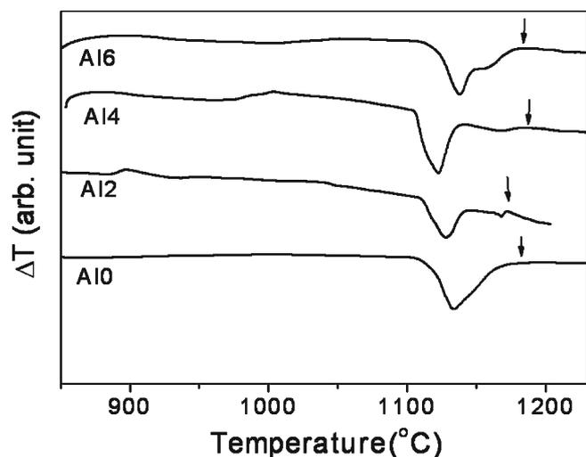
Figure 7. DTA thermograms of as cast alloys.
