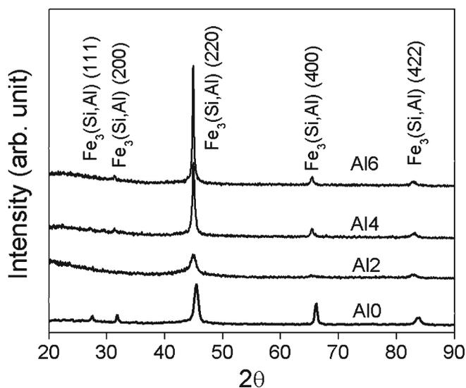
Figure 3. XRD patterns of annealed ribbons.
