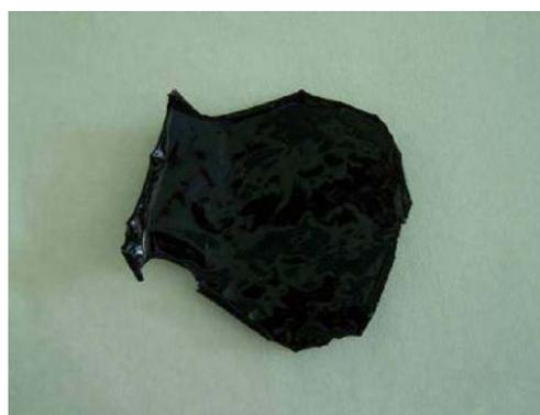
Figure 5. Photograph of SPEEK-sulfonated carbon black composite membrane.
