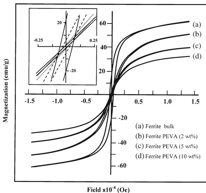
**Figure 10.** Magnetization vs field curves measured at 25 °C of bulk  $\text{Co}_{0.75}\text{Zn}_{0.25}\text{Fe}_2\text{O}_4$  and  $\text{Co}_{0.75}\text{Zn}_{0.25}\text{Fe}_2\text{O}_4/\text{PEVA}$  nanocomposite at different compositions.
