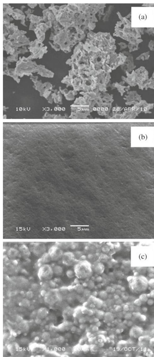
**Figure 1.** SEM images of: (a) bulk  $\text{Co}_{0.75}\text{Zn}_{0.25}\text{Fe}_2\text{O}_4$ ; (b) pure PEVA and (c)  $\text{Co}_{0.75}\text{Zn}_{0.25}\text{Fe}_2\text{O}_4$ /PEVA system with 10 wt% of ferrite content ( $C_4$ ).
