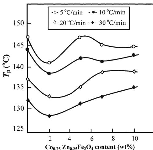
**Figure 4.** Relation between  $T_p$  (K) and composition of  $\text{Co}_{0.75}\text{Zn}_{0.25}\text{Fe}_2\text{O}_4/\text{PEVA}$  in wt%.
