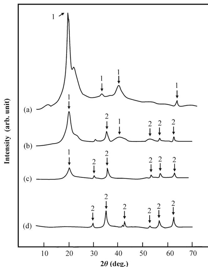
**Figure 2.** XRD patterns of: (a) pure PEVA; (b)  $\text{Co}_{0.75}\text{Zn}_{0.25}\text{Fe}_2\text{O}_4$ /PEVA (5:95 wt%)( $\text{C}_2$ ); (c)  $\text{Co}_{0.75}\text{Zn}_{0.25}\text{Fe}_2\text{O}_4$ /PEVA (10:90 wt%)( $\text{C}_4$ ) and (d) bulk  $\text{Co}_{0.75}\text{Zn}_{0.25}\text{Fe}_2\text{O}_4$  nanoparticles: line (1) PEVA and line (2)  $\text{Co}_{0.75}\text{Zn}_{0.25}\text{Fe}_2\text{O}_4$ .
