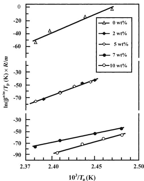
**Figure 8.** Plots of PEVA and  $\text{Co}_{0.75}\text{Zn}_{0.25}\text{Fe}_2\text{O}_4/\text{PEVA}$  (wt%) nanocomposites in accordance with Xu and Uhlmann equation.
