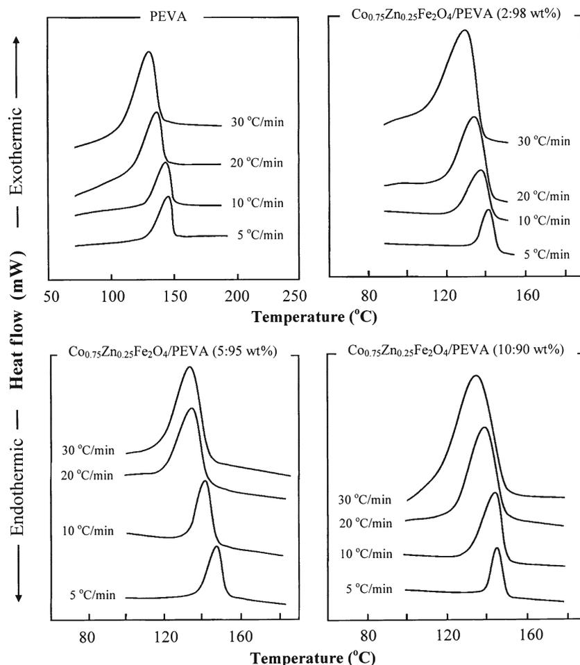
**Figure 3.** DSC thermograms at different cooling rates of pure PEVA and  $\text{Co}_{0.75}\text{Zn}_{0.25}\text{Fe}_2\text{O}_4/\text{PEVA}$  nanocomposites in wt%.
