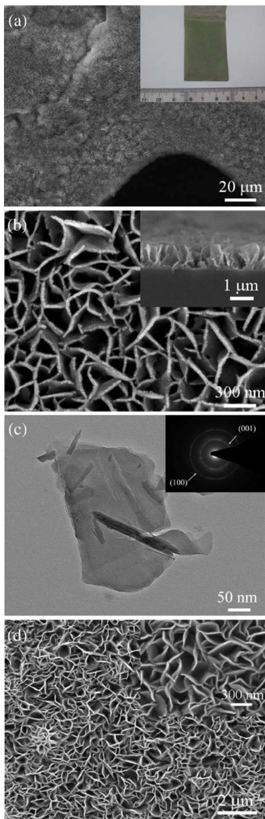
**Figure 2.** (a) and (b) SEM images of porous  $\alpha\text{-Co}(\text{OH})_2$  nanoflake array film (photograph of sample in inset); (c) TEM image of  $\alpha\text{-Co}(\text{OH})_2$  nanoflake (SAED pattern in inset) and (d) SEM image of  $\text{Co}(\text{OH})_2$  nanoflake array film after sonication for 30 min.
