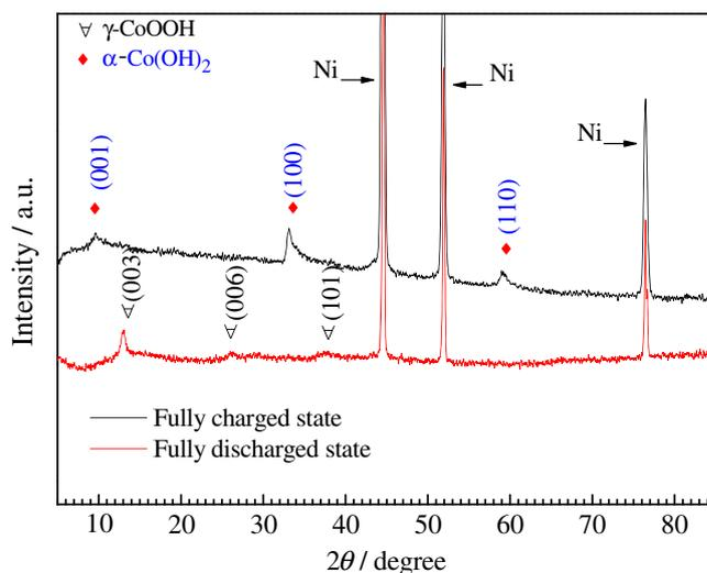
**Figure 4.** XRD patterns of porous  $\alpha\text{-Co}(\text{OH})_2$  nanoflake array film at fully charged and discharged states at 10th cycle.
