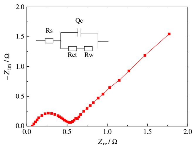
**Figure 5.** Nyquist plot of porous  $\alpha$ -Co(OH)<sub>2</sub> nanoflake array film after 100% depth of discharge at 50th cycle.
