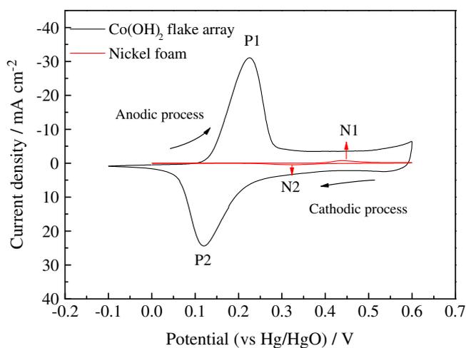
**Figure 3.** Cyclic voltammograms of porous  $\alpha\text{-Co}(\text{OH})_2$  nanoflake array film and nickel foam in potential region of  $-0.1\text{--}0.6\text{ V}$  at a scanning rate of  $10\text{ mV s}^{-1}$  at second cycle.
