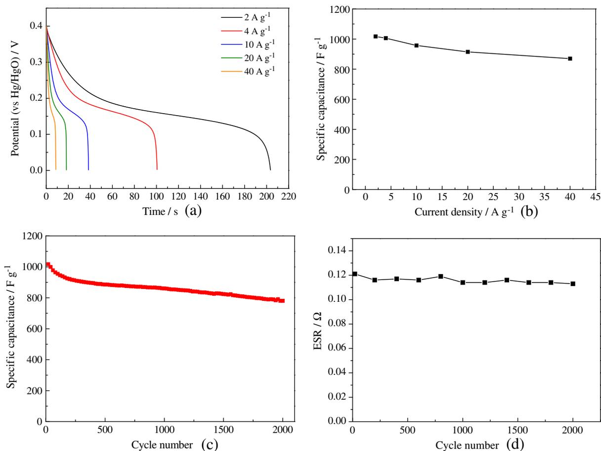
**Figure 6.** (a) Discharge curves of porous  $\alpha$ -Co(OH)<sub>2</sub> nanoflake film at different discharge current densities and (b) corresponding capacitances; (c) cycling performance of porous  $\alpha$ -Co(OH)<sub>2</sub> nanoflake array film at 2 A g<sup>-1</sup> and (d) ESR variation of ESR of porous  $\alpha$ -Co(OH)<sub>2</sub> nanoflake film with cycle number.
