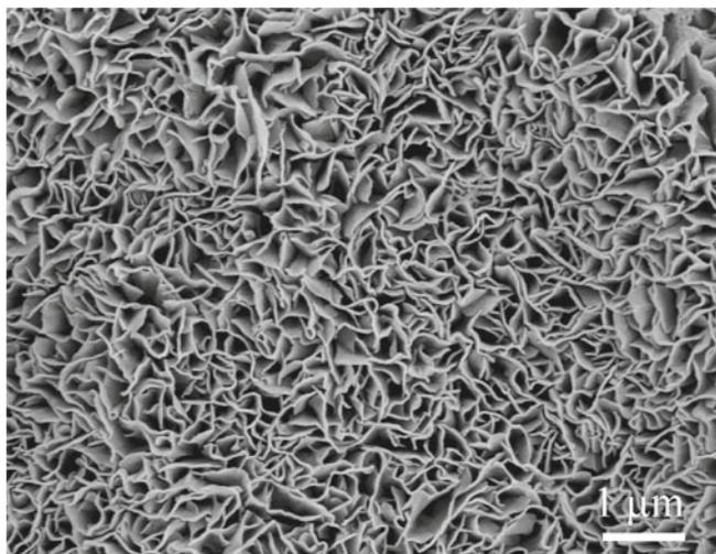
**Figure 7.** SEM image of fully discharged porous  $\alpha\text{-Co}(\text{OH})_2$  nanoflake array film after 2000 cycles.
