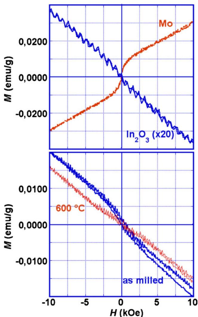
**Figure 3.** Hysteresis loop of as-received  $\text{In}_2\text{O}_3$ , Mo metal, Mo– $\text{In}_2\text{O}_3$  milled mixture and Mo– $\text{In}_2\text{O}_3$  milled mixture after annealing at 600 °C.
