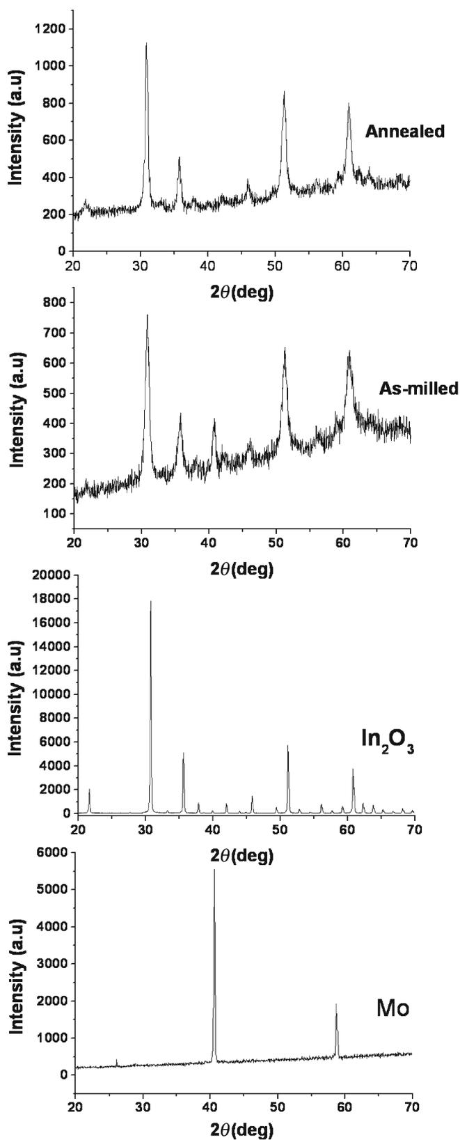
**Figure 1.** XRD patterns of as-received  $\text{In}_2\text{O}_3$ , Mo metal, Mo- $\text{In}_2\text{O}_3$  milled mixture and annealed mixture at  $600 \text{ }^\circ\text{C}$ .
