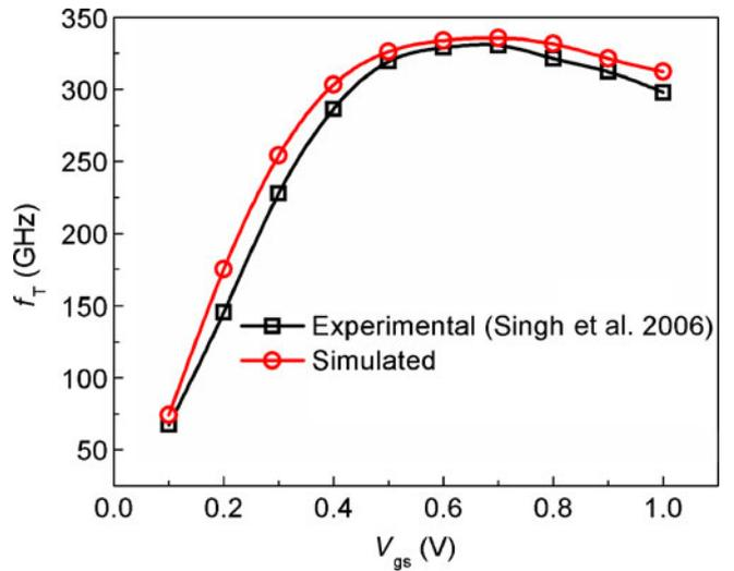
Figure 3. Comparison of gate bias dependence of  $f_T$  with experimental data of Singh *et al* (2006) and simulation for  $n$ -MOSFETs.
