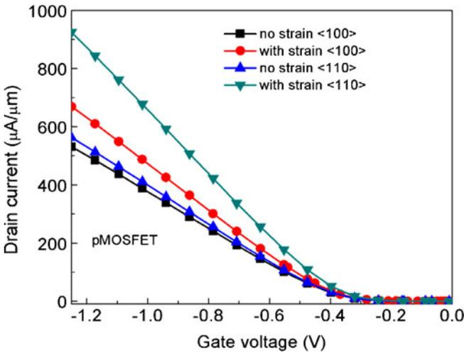
**Figure 5.** Drain current vs gate voltage ( $I_{DS} - V_{GS}$ ) characteristics for  $p$ -MOS devices with and without compressive stress.
