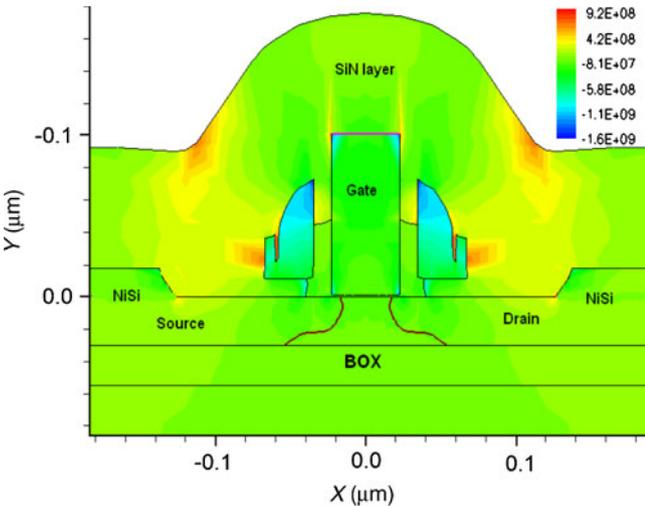
Figure 2. Stress distribution ( $y$  component) of stress tensor ( $\sigma_{yy}$ ) in device at end of process flow.
