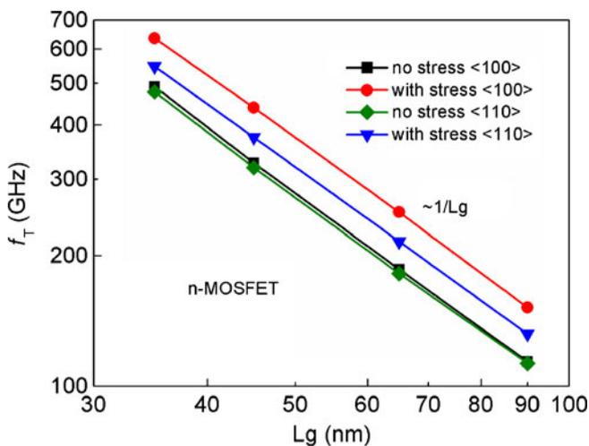
**Figure 6.**  $f_T$  vs gate length for different orientations for  $n$ -MOSFETs.
