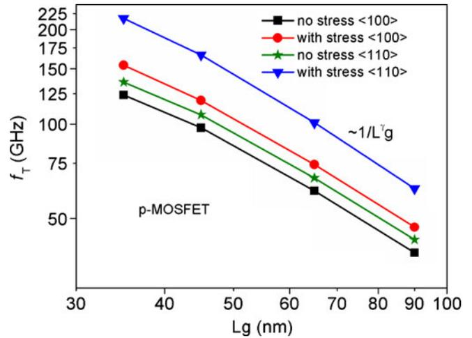
**Figure 7.**  $f_T$  vs gate length for different orientations for  $p$ -MOSFETs.
