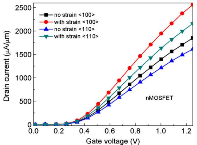
Figure 4. Comparison of  $I_{DS} - V_{GS}$  characteristics for devices with a highly tensile cap layer and a relaxed cap layer.
