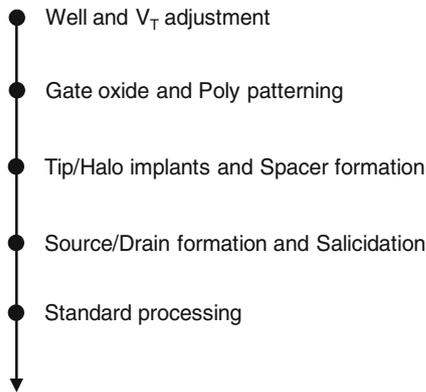
Figure 1. Typical process flow used in simulation.
