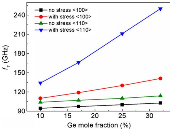
**Figure 9.** Variation of  $f_T$  as a function Ge mole fraction in  $p$ -MOSFETs.
