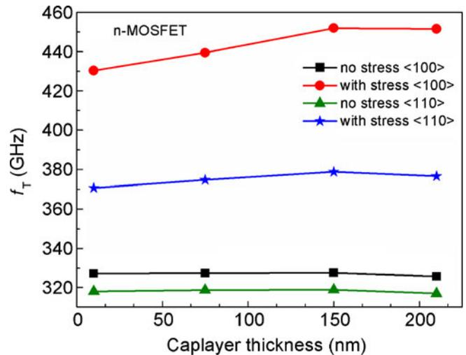
**Figure 8.** Effect of cap layer thickness on  $f_T$  for various channels stress condition in  $n$ -MOSFETs.
