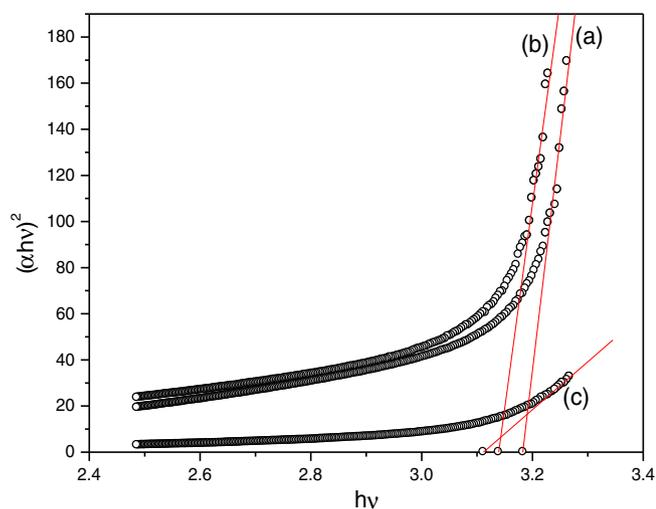
**Figure 6.** Photon energy (eV) dependence of (a) ZnO, (b) 5% Cd:ZnO and (c) 10% Cd:ZnO.
