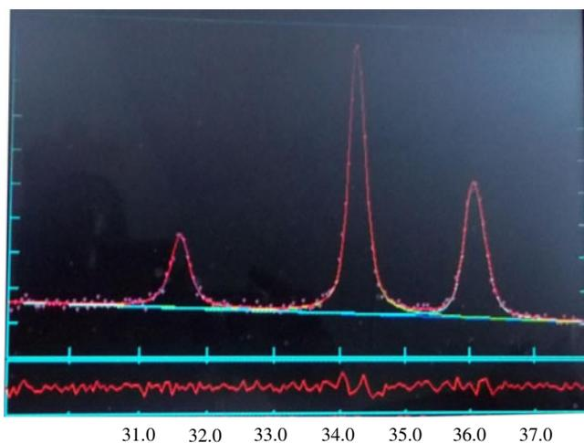
**Figure 2.** Observed (dotted) and simulated (continuous) X-ray diffraction patterns of ZnO.
