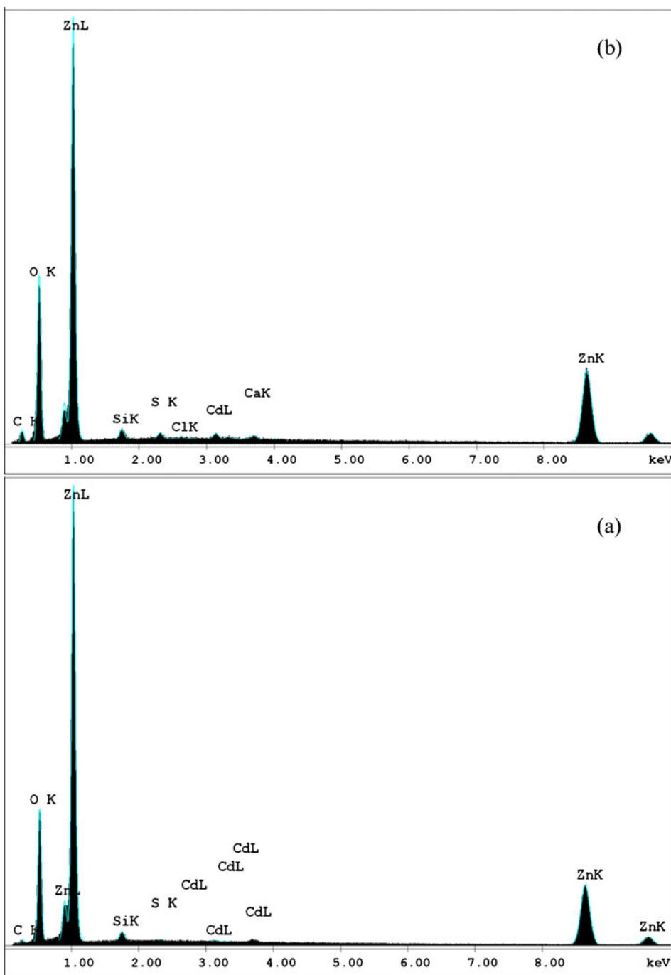
Figure 5. EDX pattern of (a) 5% Cd:ZnO and (b) 10% Cd:ZnO.
