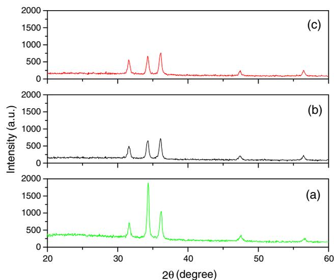
**Figure 1.** X-ray diffraction patterns of (a) 0 ZnO, (b) 5% Cd-doped ZnO and (c) 10% Cd-doped ZnO.
