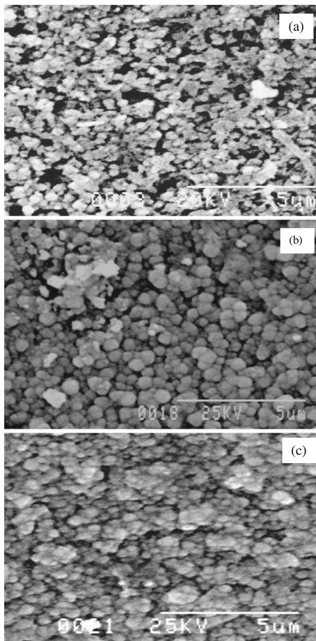
**Figure 4.** SEM images of (a) undoped ZnO, (b) 5% Cd:ZnO and (c) 10% Cd:ZnO.
