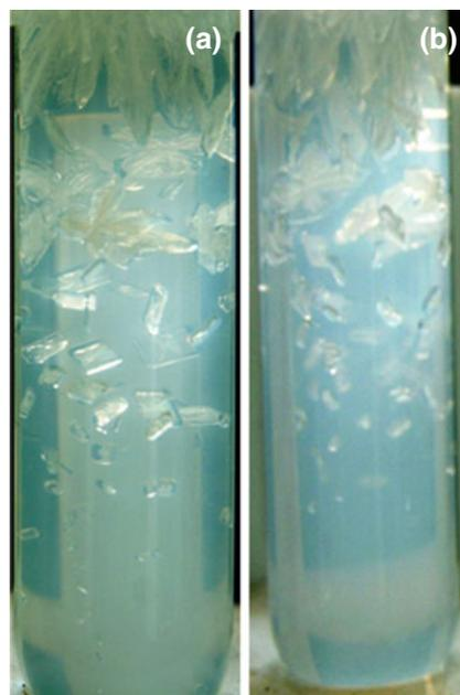
Figure 1. MAP crystals in tubes a. pure and b. 0.3 M NaF.
