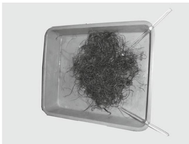
**Figure 2.** Treated coir fibres.
