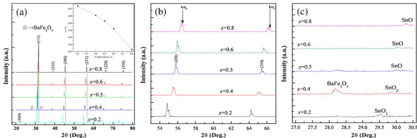
**Figure 1.** XRD patterns of  $\text{Sr}_x\text{Ba}_{1-x}\text{Fe}_{0.6}\text{Sn}_{0.4}\text{O}_{3-\varepsilon}$  sintered at  $1280\text{--}1300^\circ\text{C}$  for 2 h. Inset represents lattice parameter,  $a$  evolution vs compositions ( $x$ ) in the system of  $\text{Sr}_x\text{Ba}_{1-x}\text{Fe}_{0.6}\text{Sn}_{0.4}\text{O}_{3-\varepsilon}$ .
