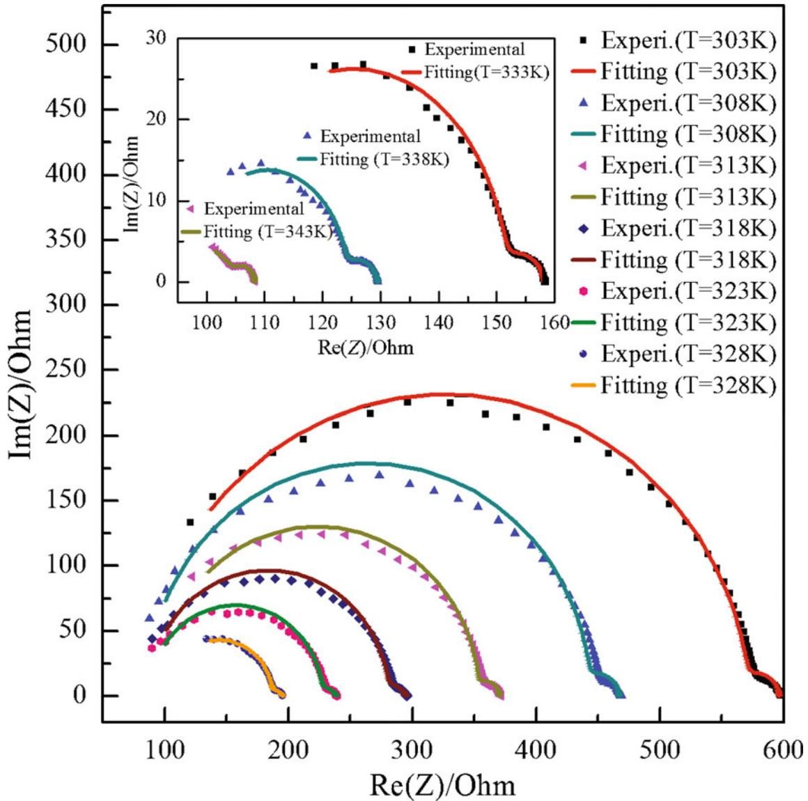
**Figure 5.** Impedance diagrams of  $\text{Sr}_{0.4}\text{Ba}_{0.6}\text{Fe}_{0.6}\text{Sn}_{0.4}\text{O}_{3-\varepsilon}$  ceramic at different temperatures.
