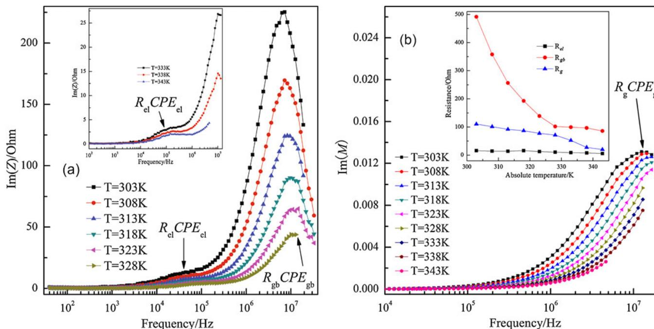
**Figure 6.** Variation of (a)  $\text{Im}(Z)$  and (b)  $\text{Im}(M)$  with frequency at different temperatures for composition  $x = 0.4$ . Inset of figure 6(b) shows values of resistance  $R_{gb}$ ,  $R_g$  and  $R_{el}$ , as a function of absolute temperature,  $T$ .
