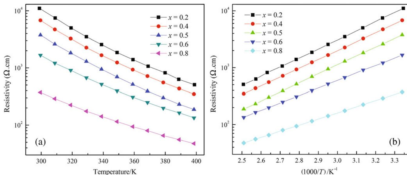
**Figure 3.** (a) Relationship between electrical resistivity ( $\rho$ ) and absolute temperature ( $T$ ) for  $\text{Sr}_x\text{Ba}_{1-x}\text{Fe}_{0.6}\text{Sn}_{0.4}\text{O}_{3-\varepsilon}$  ( $0.2 \leq x \leq 0.8$ ) ceramics and (b) relationship between logarithmic  $\rho$  and reciprocal of absolute temperature ( $1/T$ ) for  $\text{Sr}_x\text{Ba}_{1-x}\text{Fe}_{0.6}\text{Sn}_{0.4}\text{O}_{3-\varepsilon}$  ( $0.2 \leq x \leq 0.8$ ) ceramics.
