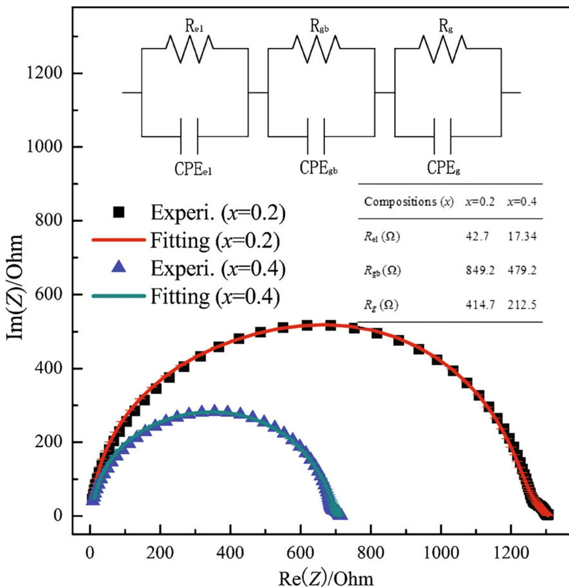
**Figure 4.** Impedance diagrams of  $\text{Sr}_x\text{Ba}_{1-x}\text{Fe}_{0.6}\text{Sn}_{0.4}\text{O}_{3-\varepsilon}$  ( $x = 0.2$  and  $0.4$ ) samples at 298 K. Inset represents equivalent circuit model.
