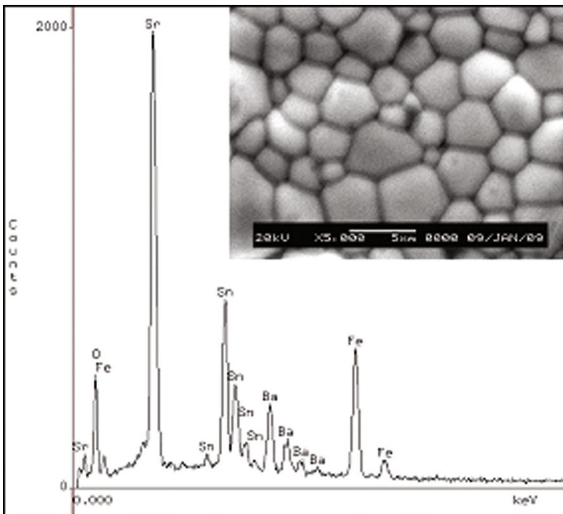
**Figure 2.** EDS spectra of composition,  $x = 0.8$ . Inset shows SEM microphotograph of  $Sr_{0.8}Ba_{0.2}Fe_{0.6}Sn_{0.4}O_{3-\varepsilon}$  ceramic.
