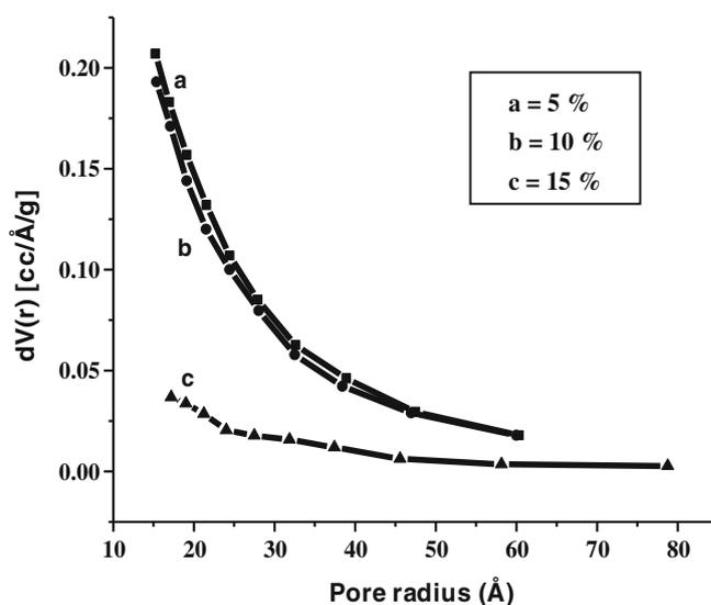
**Figure 8.** BJH plot of  $Zn_{1-x}Mn_xO$  nanoparticles for  $x =$  (a) 0.05, (b) 0.10 and (c) 0.15 heated at 700°C.
