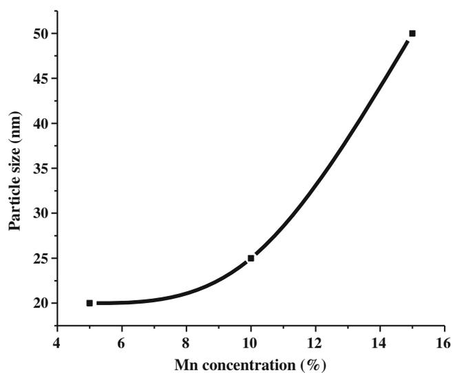
**Figure 5.** Plot of variation of particle size vs manganese concentration.
