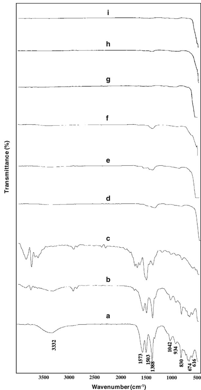
**Figure 3.** FTIR spectrum of  $Zn_{1-x}Mn_xO$  nanoparticles for  $x =$  (a) 0.05, (b) 0.10, (c) 0.15 at room temperature, (d) 0.05, (e) 0.10, (f) 0.15 heated at  $500^\circ\text{C}$ , (g) 0.05, (h) 0.10 and (i) 0.15 heated at  $700^\circ\text{C}$ .
