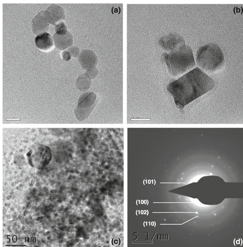
**Figure 4.** TEM micrographs of  $Zn_{1-x}Mn_xO$  solid solution at (a)  $x = 0.05$ , (b)  $x = 0.10$  and (c)  $x = 0.15$ , and (d) SAED of  $Zn_{0.85}Mn_{0.15}O$  nanoparticles.
