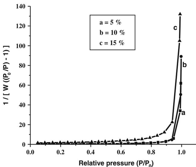
**Figure 7.** BET plot of  $Zn_{1-x}Mn_xO$  nanoparticles for  $x =$  (a) 0.05, (b) 0.10 and (c) 0.15 heated at 700°C.
