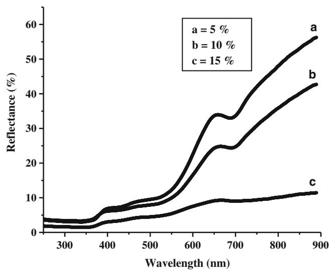
**Figure 6.** UV-visible reflectance spectra of  $Zn_{1-x}Mn_xO$  nanoparticles for  $x =$  (a) 0.05, (b) 0.10 and (c) 0.15 heated at  $700^\circ\text{C}$ .
