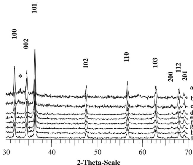
**Figure 2.** Powder X-ray diffraction pattern of  $Zn_{1-x}Mn_xO$  nanoparticles for  $x =$  (a) 0.05, (b) 0.10, (c) 0.15 at room temperature, (d) 0.05, (e) 0.10, (f) 0.15 heated at  $500^\circ\text{C}$ , (g) 0.05, (h) 0.15 and (i) 0.10 heated at  $700^\circ\text{C}$ .
