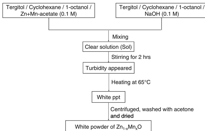
**Figure 1.** Flowchart for reverse micellar synthesis of Mn-doped ZnO nanoparticles.
