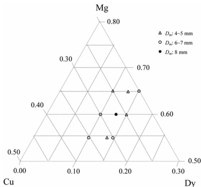
**Figure 1.** The alloy compositions for forming BMGs studied in the Mg-Cu-Dy system.
