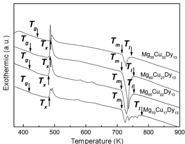
**Figure 3.** DSC traces of the as-cast Mg<sub>x</sub>Cu<sub>y</sub>Dy<sub>13</sub> BMGs with a heating rate of 0.67 K/s.
