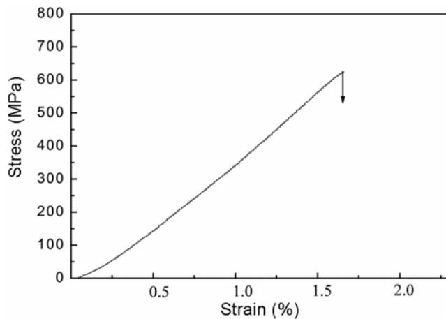
**Figure 4.** The Stress–strain curve of  $\text{Mg}_{60}\text{Cu}_{27}\text{Dy}_{13}$  BMG.
