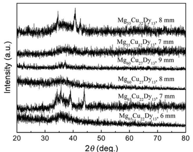
**Figure 2.** XRD patterns obtained from the as-cast rods with different diameters for  $Mg_xCu_yDy_{13}$  alloys.
