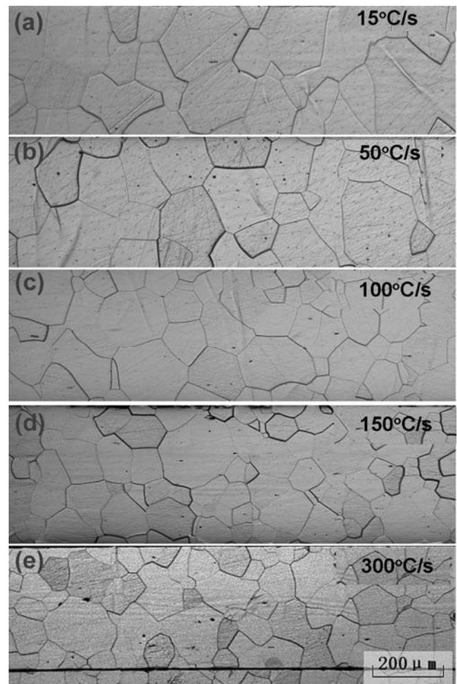
**Figure 2.** Optical microstructures of recrystallized specimens with different heating rates (100×). (a) 15°C/s; (b) 50°C/s; (c) 100°C/s; (d) 150°C/s and (e) 300°C/s.
