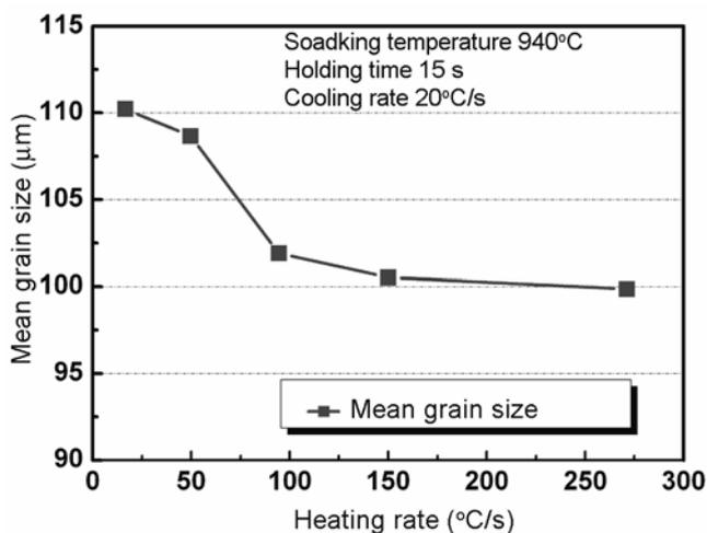
Figure 3. Mean grain-size as a function of annealing heating rates.
