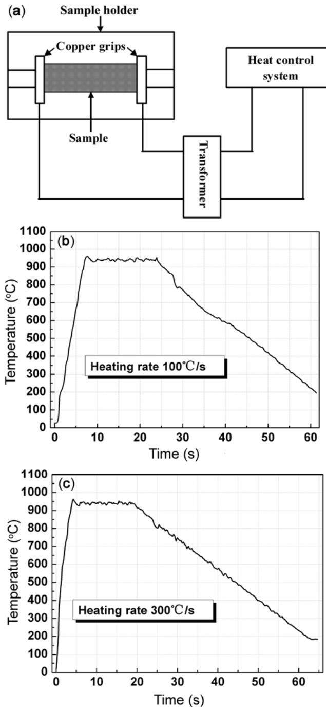
**Figure 1.** (a) Scheme of rapid heating experimental setup, (b) thermal cycle of treated samples with 100°C/s, (c) thermal cycle of treated samples with 300°C/s.
