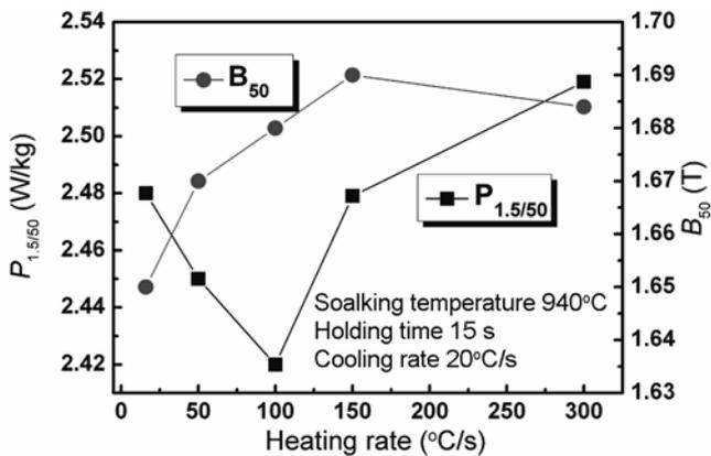
Figure 6. Effect of heating rates on core loss ( $P_{1.5/50}$ ) and magnetic induction ( $B_{50}$ ) for samples.
