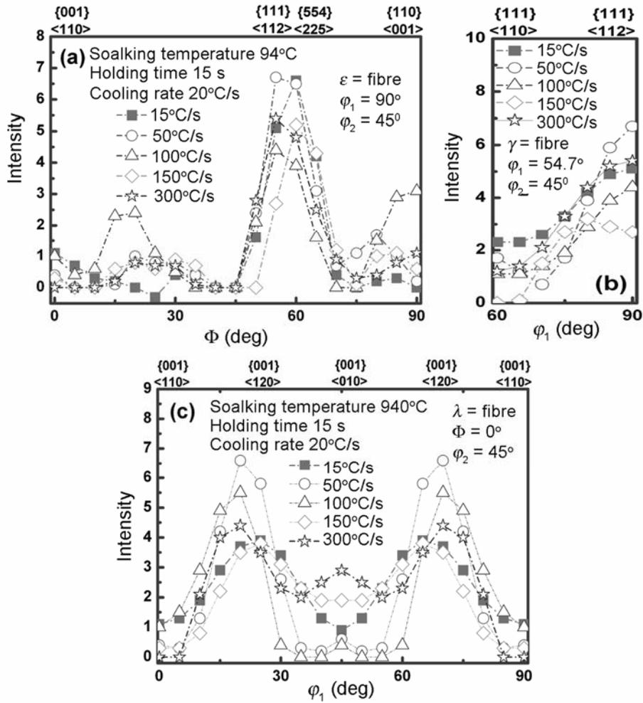
Figure 5. Intensity of different fibre texture in samples with different heating rates: (a)  $\epsilon$ -fibre texture; (b)  $\gamma$ -fibre texture and (c)  $\lambda$ -fibre texture.
