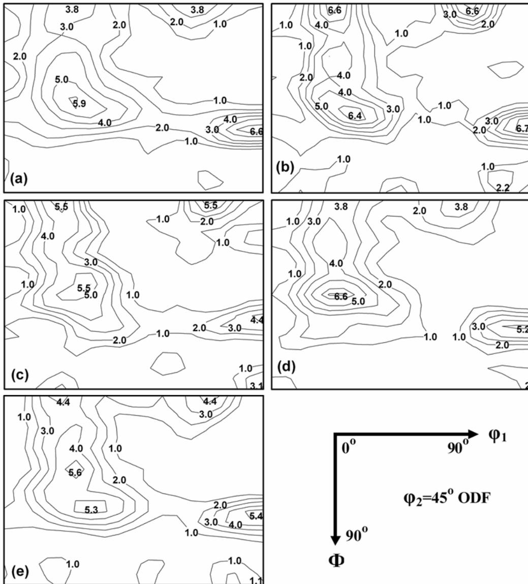
**Figure 4.** The  $\varphi_2 = 45^\circ$  section of Euler space using the Bunge angular convention with different heating rates. (a) 15°C/s; (b) 50°C/s; (c) 100°C/s; (d) 150°C/s and (e) 300°C/s.
