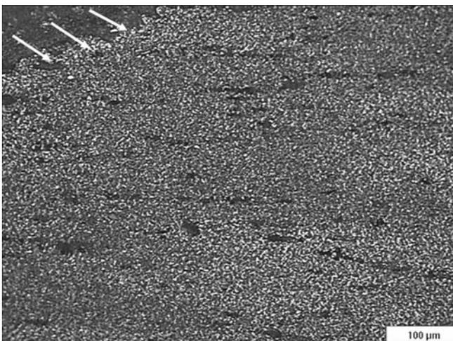
Figure 9. Microstructure of gauge surface, obtained by optical microscopy, for sample that gave highest ductility. The arrows point at fractured surface of tensile specimen.
