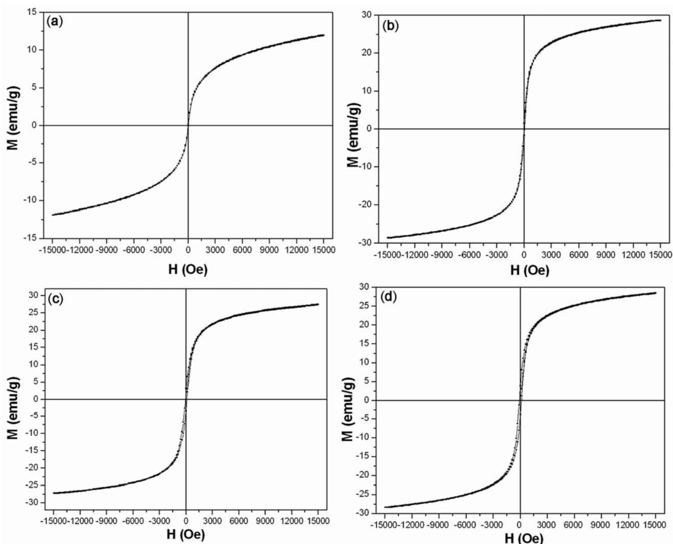
**Figure 5.** Room temperature hysteresis loop of  $\text{NiFe}_2\text{O}_4$  nanoparticles prepared by (a) co-precipitation, annealed at  $400^\circ\text{C}$ , (b) co-precipitation, annealed at  $600^\circ\text{C}$ , (c) sol-gel technique, annealed at  $400^\circ\text{C}$  and (d) sol-gel technique, annealed at  $600^\circ\text{C}$ .
