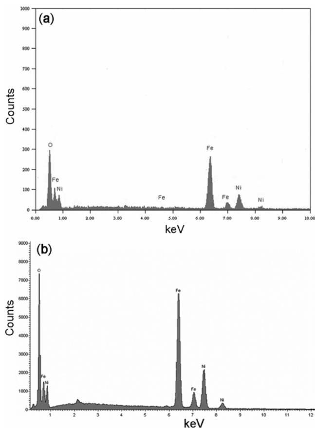
**Figure 2.** EDX spectra of NiFe<sub>2</sub>O<sub>4</sub> nanoparticles prepared by (a) co-precipitation and (b) sol-gel technique.
