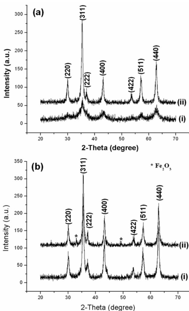
**Figure 1.** X-ray diffraction patterns of  $\text{NiFe}_2\text{O}_4$  nanoparticles prepared by (a) co-precipitation, annealed at (i)  $400^\circ\text{C}$  and (ii)  $600^\circ\text{C}$  and (b) sol-gel, annealed at (i)  $400^\circ\text{C}$  and (ii)  $600^\circ\text{C}$ .
