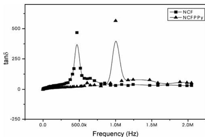
**Figure 4.** Variation of the loss tangent ( $\tan \delta$ ) as a function of frequency for pristine NCF and NCFPPy samples at 300 K.
