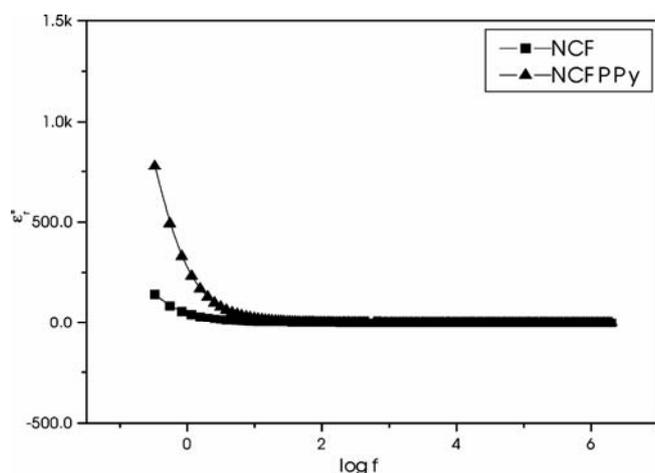
**Figure 3.** Variation of the numerical value of dielectric loss ( $\epsilon''_r$ ) as a function of log frequency for pristine NCF and NCFPPy samples at 300 K.
