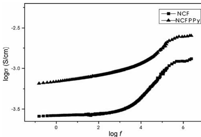
**Figure 5.** Variation of the logarithmic conductivity with log frequency of pristine NCF and NCFPPy samples at 300 K.
