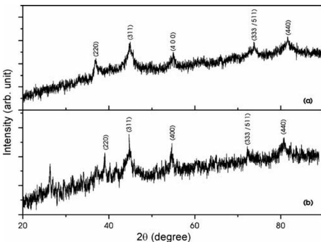
**Figure 1.** X-ray diffraction patterns of (a) pristine NCF nanoparticles and (b) NCFPPy nanocomposite.
