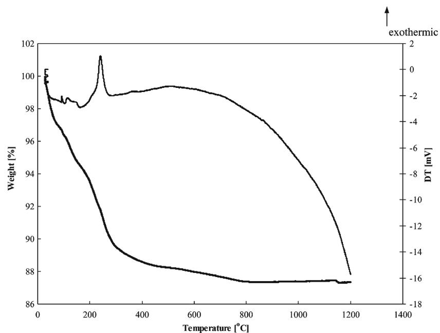
**Figure 8.** TG-DTA curves of titania powder aged at 130 °C for 12 h (second aging stage).
