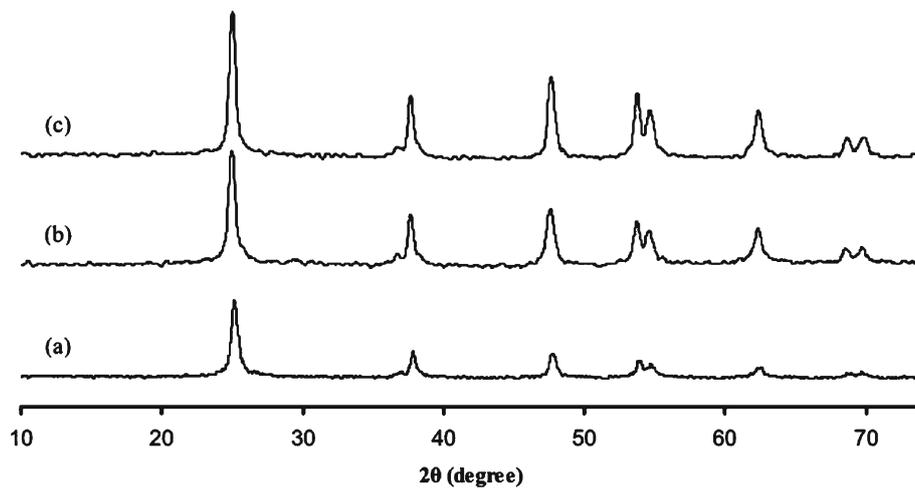
Figure 4. XRD pattern of titanium dioxide aged at 130°C for (a) 4, (b) 8 and (c) 12 h.
