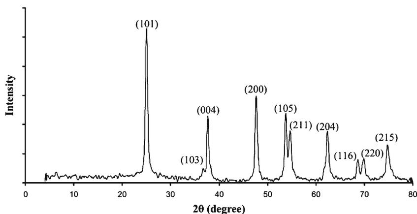
Figure 3. XRD pattern of titania powder produced after aging for 12 h at  $130^\circ C$  (second aging stage).
