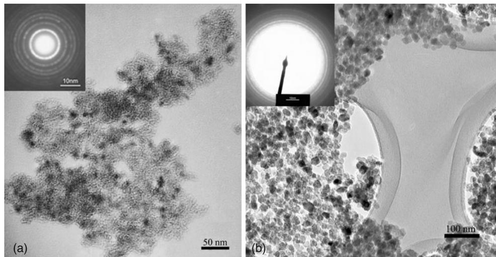
**Figure 7.** Bright field TEM images of nanoparticles aged at (a) 130 °C for 8 h and (b) 150 °C for 12 h. Insets are diffraction patterns of powders.
