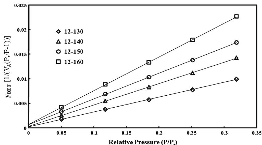
Figure 5. N<sub>2</sub> adsorption of BET plot of titanium dioxide powders heat treated at 130, 140, 150 and 160°C for 12 h.
