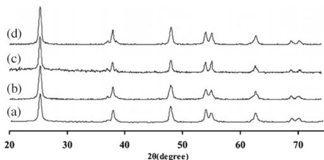
**Figure 6.** XRD patterns of titanium dioxide powders aged for 12 h at (a) 130, (b) 140, (c) 150 and (d) 160°C.
