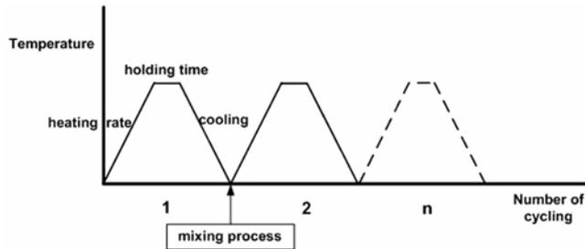
**Figure 1.** Schematic cycling synthesis.
