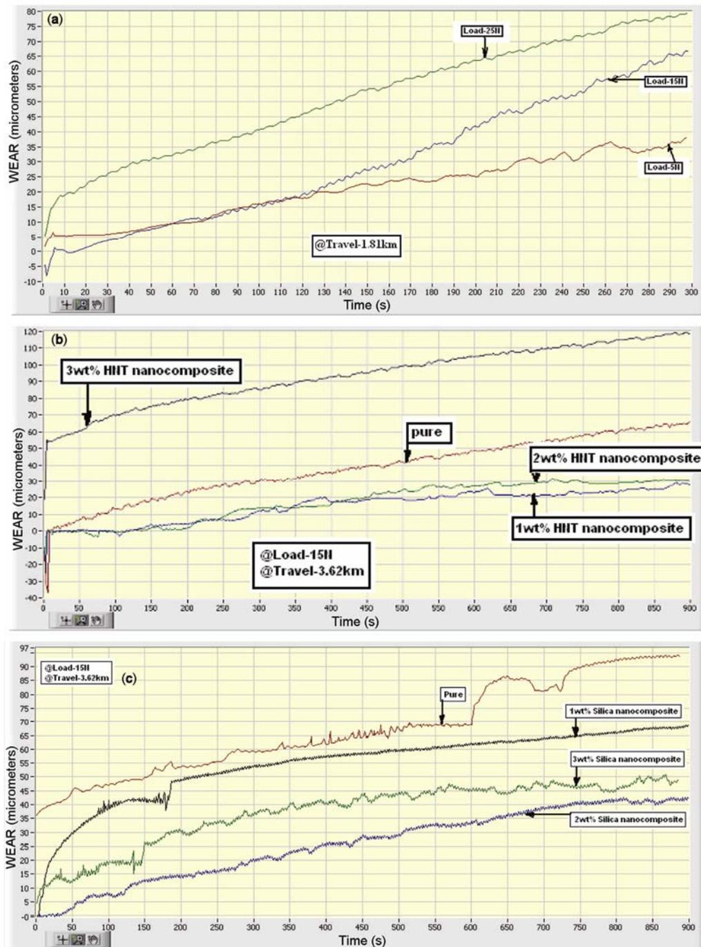
**Figure 13.** (a) Wear of pure polymer composite with load changes from 5–25 N. (b) Wear at load 5N and track distance 3.64 km for pure, 1% HNT NC, 2% HNT NC and 3% HNT NC. (c) Wear at load 15 N and track distance 3.62 km for pure, 1% NS, 2% NS and 3% NS.
