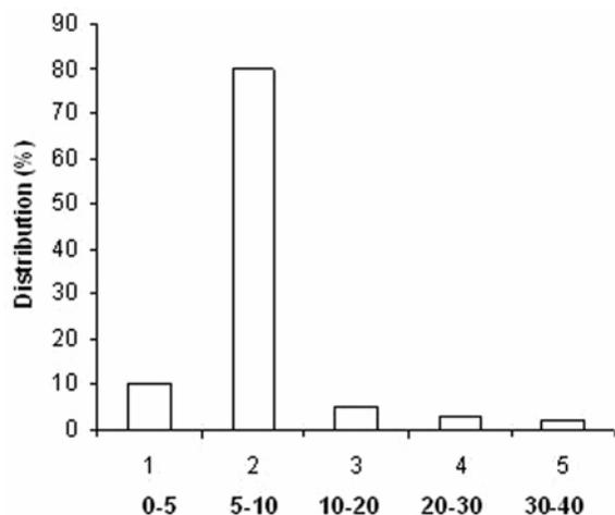
Figure 3. Distribution (%) of silver nanoparticles (nm).
