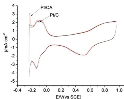
Figure 3. Cyclic voltammetry curves of Pt/CA catalyst and Pt/C catalyst (JM) in 0.5 mol/L H<sub>2</sub>SO<sub>4</sub> solution.
