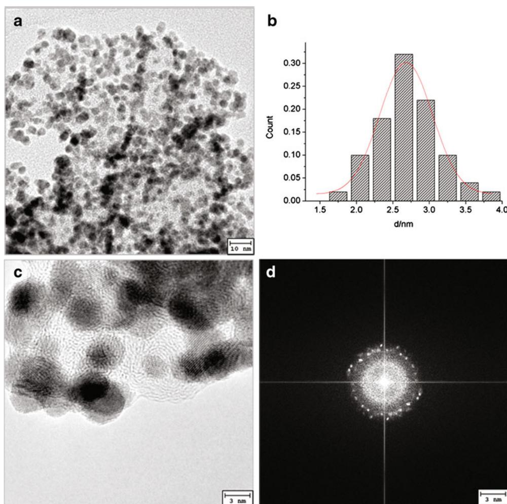
**Figure 1.** (a) and (c) HRTEM images; (b) histograms of particle size distribution; and (d) electron diffraction pattern of a region of Pt/CA catalyst.
