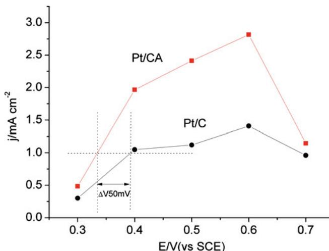
**Figure 6.** Potential-dependent steady-state current density of methanol oxidation on Pt/CA catalyst and Pt/C catalyst (JM).
