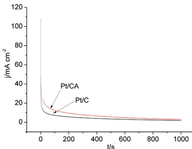
**Figure 5.** Chronoamperometry curves of Pt/CA catalyst and Pt/C catalyst (JM) in  $0.5 \text{ mol/L H}_2\text{SO}_4 + 0.5 \text{ mol/L CH}_3\text{OH}$  solution.
