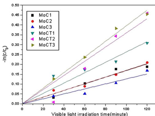
**Figure 6.** Apparent first-order linear transform  $-\ln(c/c_0)$  against irradiation time of MB degradation kinetic plots for Mo–C and Mo–CT composites.
