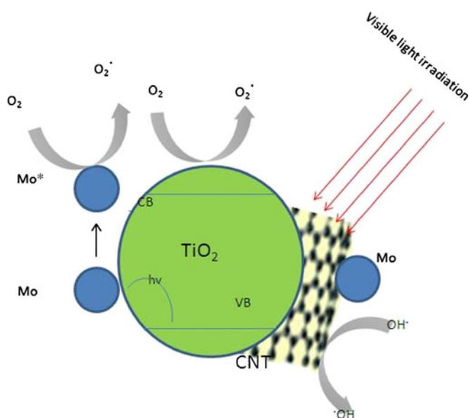
**Figure 7.** Proposed redox mechanism of Mo-CNT/TiO<sub>2</sub> composites under visible-light irradiation.
