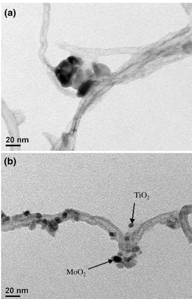
**Figure 4.** TEM micrographs obtained from powdered Mo-CNT and Mo-CNT/TiO<sub>2</sub> composites. (a) MoC3 and (b) MoCT3.
