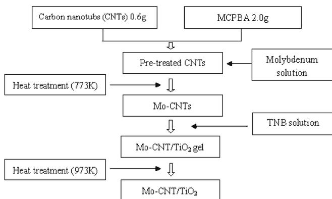
**Figure 1.** Flow chart of fabrication of Mo-CNT/TiO<sub>2</sub> composites.
