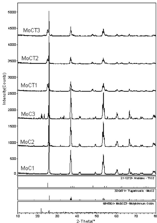
**Figure 2.** XRD patterns of Mo-CNT/TiO<sub>2</sub> composites.
