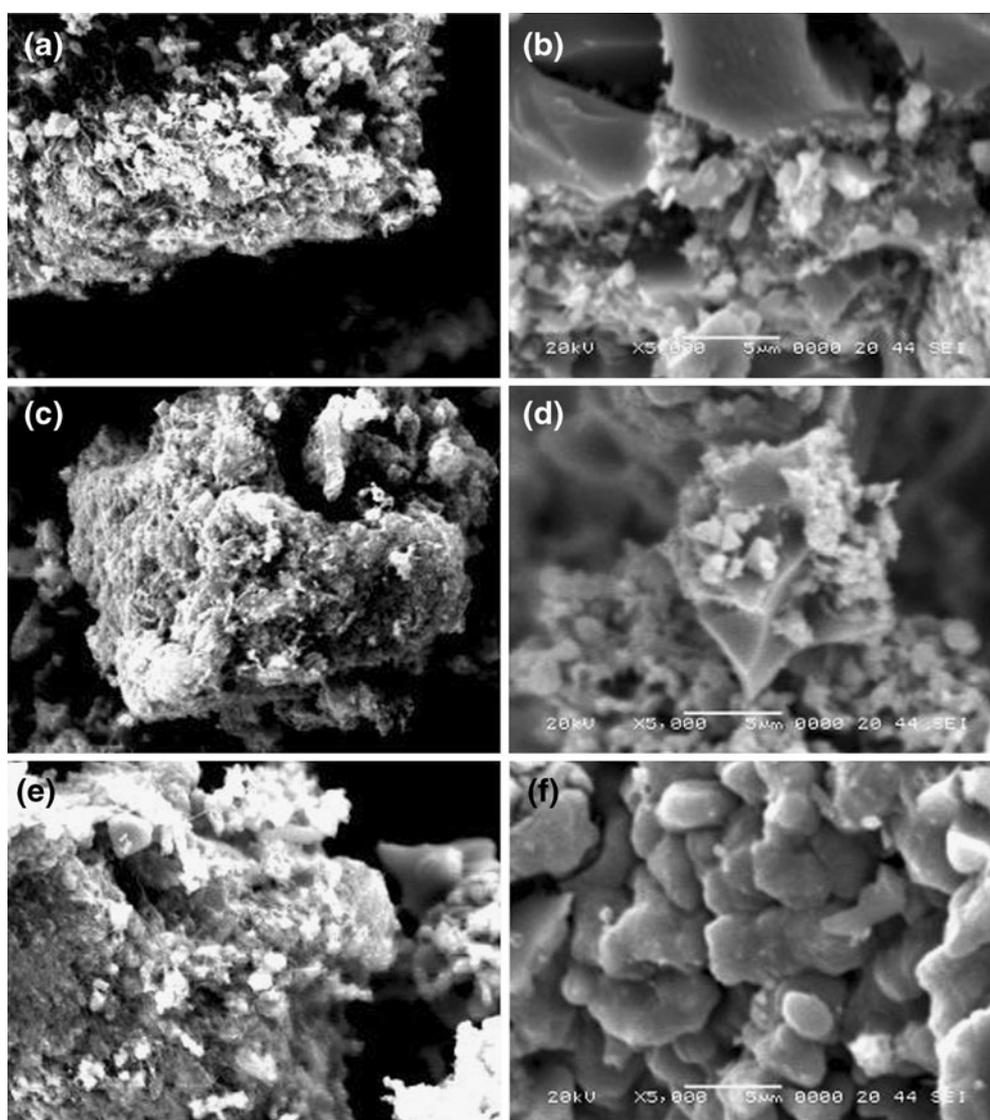
**Figure 3.** SEM images obtained from powdered Mo–CNT and Mo–CNT/TiO<sub>2</sub> composites. (a) MoC1, (b) MoCT1, (c) MoC2, (d) MoCT2, (e) MoC3 and (f) MoCT3.
