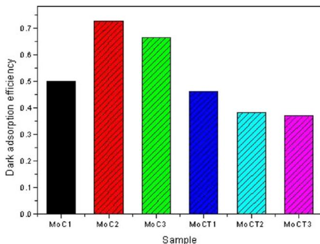
**Figure 5.** Dark adsorption efficiency of MoC and MoCT composites for MB degradation.
