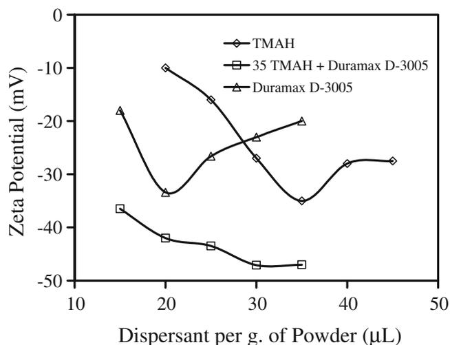
**Figure 4.** Change in zeta potentials of treated MAS powders in water as a function of dispersant concentration in the suspension.
