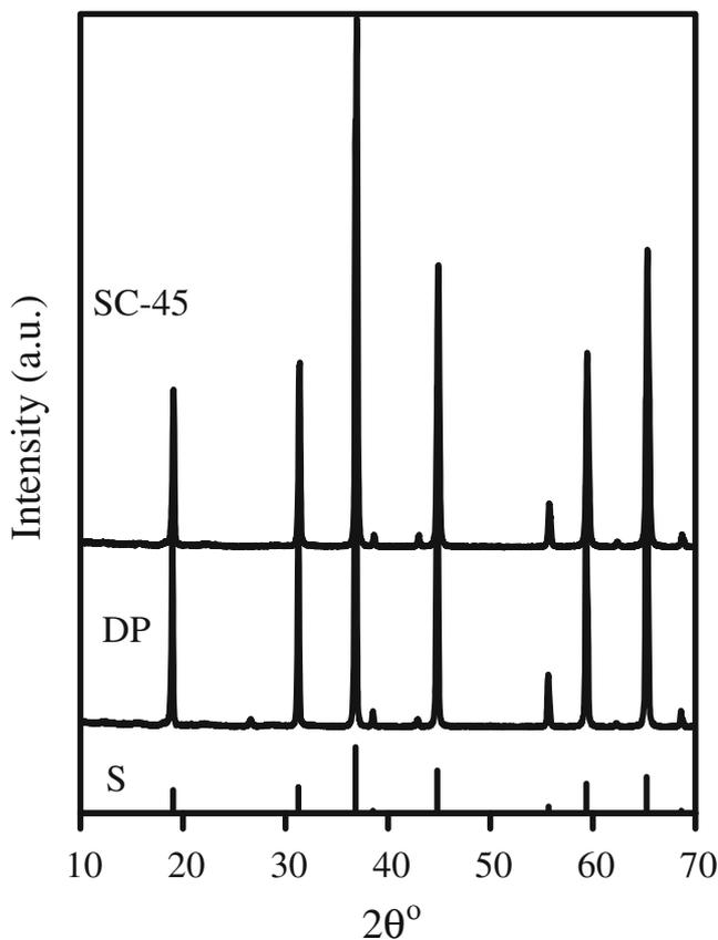
**Figure 6.** XRD patterns of DP and SC-45 consolidated bodies sintered for 1 h at 1650°C and 2 h at 1600°C, respectively. S, spinel, ICDD File No. 00-21-1152.
