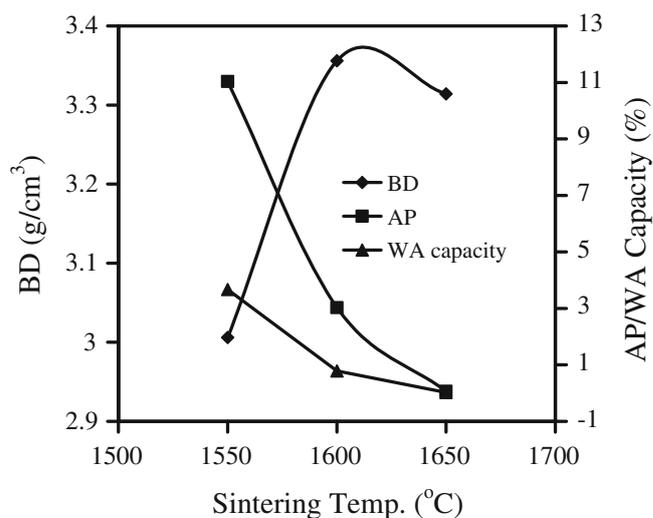
**Figure 5.** Evolution of bulk density (BD), apparent porosity (AP) and water absorption (WA) capacity of  $MgAl_2O_4$  spinel consolidated by slip casting route using aqueous suspension containing 45 vol.% solids and sintered for 2 h at 1550–1650°C.
