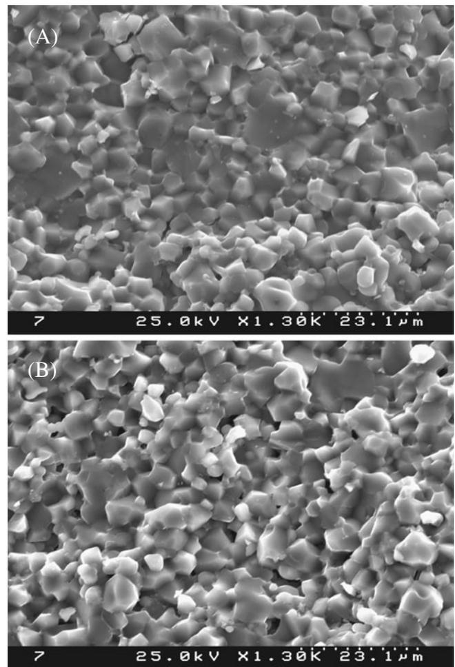
**Figure 7.** SEM micrographs of fracture surfaces of DP and SC-45 consolidated bodies sintered for 1 h at 1650°C and 2 h at 1600°C, respectively.
