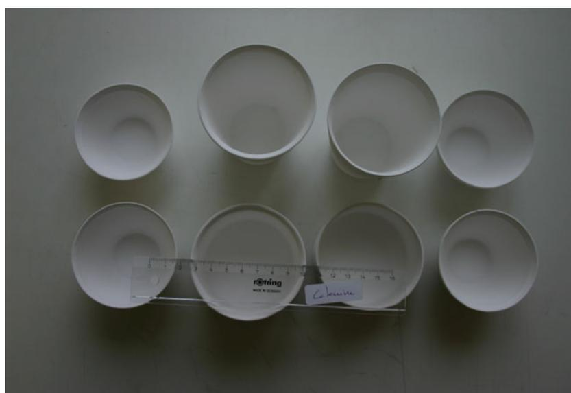
**Figure 1.** Green  $MgAl_2O_4$  spinel crucibles consolidated by aqueous slip casting from a suspension containing 45 vol.% solids loading.
