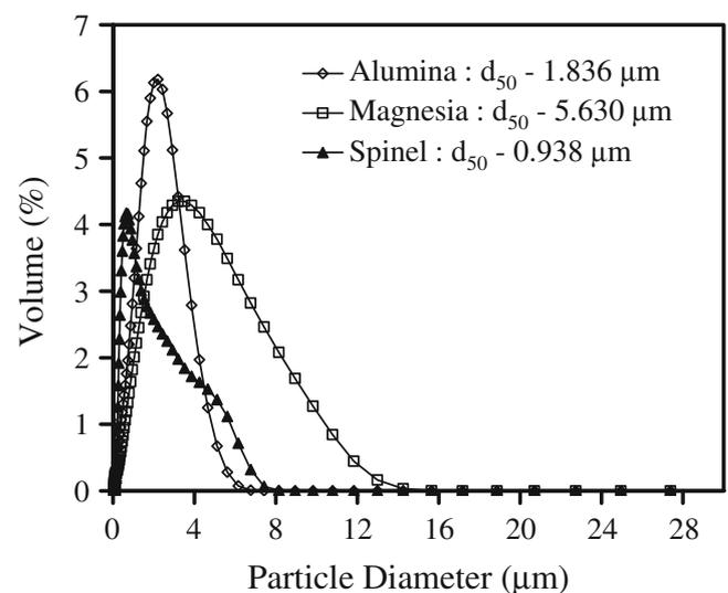
**Figure 2.** Particle size distributions of as purchased  $\alpha\text{-Al}_2\text{O}_3$  and calcined caustic MgO powders, and of the planetary ball milled  $\text{MgAl}_2\text{O}_4$  spinel formed at  $1400^{\circ}\text{C}$  for  $1\ \text{h}$ .
