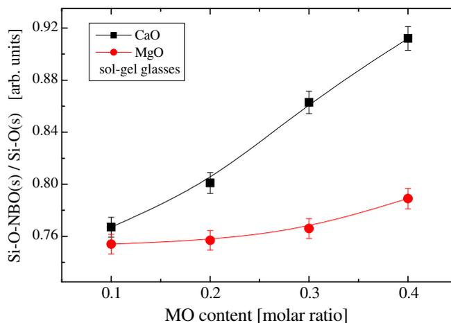
**Figure 4.** Si–O–NBO(s)/Si–O(s) absorbance intensity ratio versus modifier composition for the  $x\text{MO}\cdot(1-x)\text{SiO}_2$  ( $M = \text{Ca}, \text{Mg}$ ) glasses. Lines are drawn as guide to the eye.
