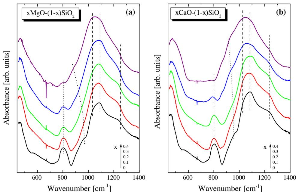
**Figure 3.** IR absorbance spectra of the binary glassy systems: (a)  $x\text{MgO}\cdot(1-x)\text{SiO}_2$  and (b)  $x\text{CaO}\cdot(1-x)\text{SiO}_2$  ( $x = 0, 0.1, 0.2, 0.3$  and  $0.4$ ) prepared by sol-gel technique at room temperature.
