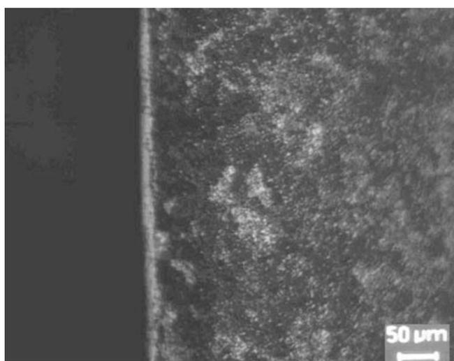
**Figure 5.** Microstructural view of plasma nitrided annealed sample for 25% nitrogen and 75% argon gas compositions and at 200 magnification.
