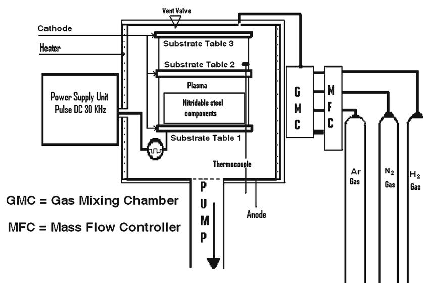
Figure 1. Block diagram of the plasma nitriding system.
