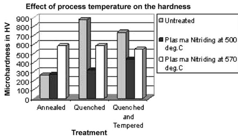
**Figure 2.** Effect of the process temperature on the hardness of AISI 52100 steel subjected to different heat treatments. Shaded bar shows the hardness of untreated samples, dark bar shows the hardness of plasma nitrided samples at 500°C and bright bar shows the hardness of the plasma nitrided samples at 570°C.
