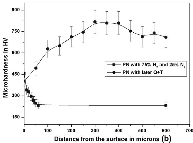
**Figure 8.** Microhardness depth profile of annealed sample after plasma nitriding and also with later heat treatment. (a) 25% Nitrogen and 75% argon gas and (b) 25% nitrogen and 75% hydrogen gas.
