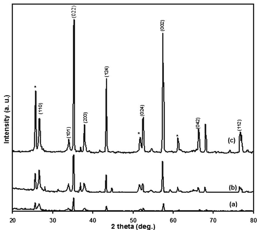
**Figure 3.** XRD patterns of  $\text{SnO}_2$  thin films annealed at (a)  $550^\circ\text{C}$ , (b)  $750^\circ\text{C}$  and (c)  $950^\circ\text{C}$ .
