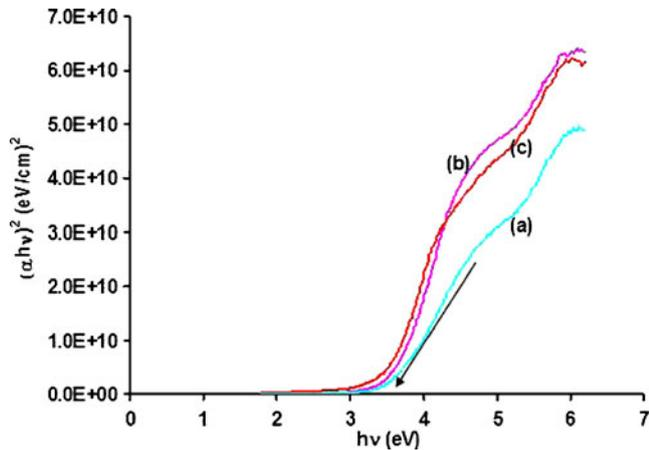
**Figure 6.** Plot of  $(\alpha hv)^2$  vs photon energy ( $hv$ ) for the annealing temperatures (a) 550°C, (b) 750°C and (c) 950°C.
