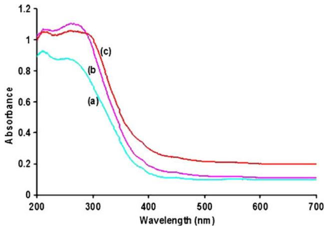
**Figure 5.** Variation of absorbance with wavelength ( $\lambda$ ), nm, for annealing temperatures (a) 550°C, (b) 750°C and (c) 950°C.
