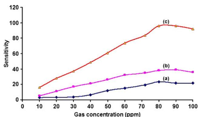
**Figure 8.** Dependence of the sensitivity of the SnO<sub>2</sub> on H<sub>2</sub>S concentration at 100°C.
