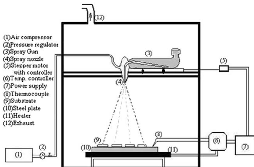
Figure 1. Schematic representation of the spray system.
