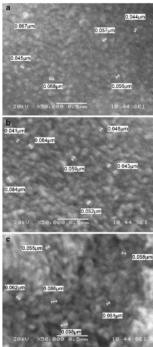
**Figure 4.** SEM photographs at annealing temperatures (a) 550°C, (b) 750°C and (c) 950°C.
