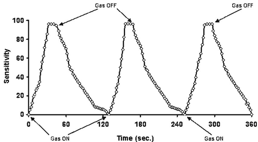
Figure 10. Response and recovery of the SnO<sub>2</sub> film.
