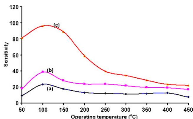
**Figure 7.** Effect of annealing temperature on the sensitivity of SnO<sub>2</sub> thin films at (a) 550°C, (b) 750°C and (c) 950°C to 80 ppm of H<sub>2</sub>S gas.
