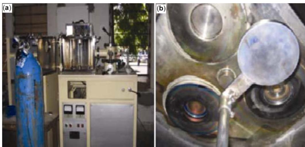
**Figure 1.** Sputtering unit with multiple targets. (a) View of sputtering unit with Argon cylinder and (b) direct sputtering with three target and substrate holders.
