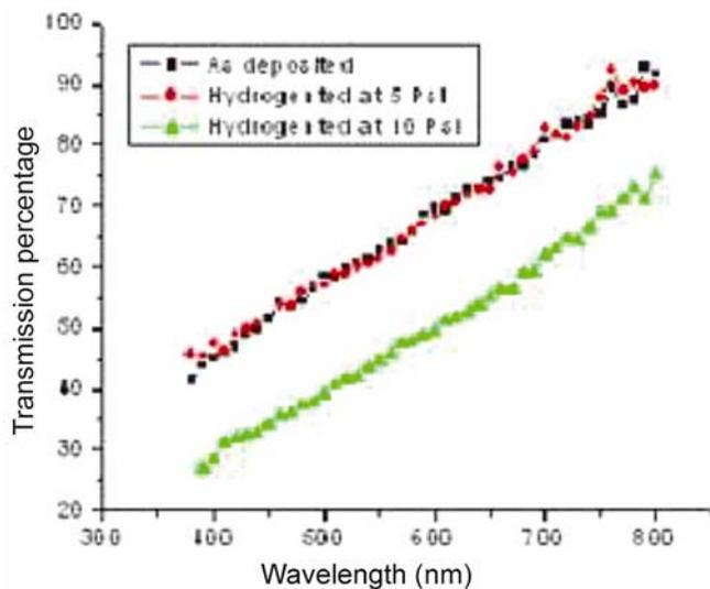
Figure 3. Transmission spectra of tantalum thin films.
