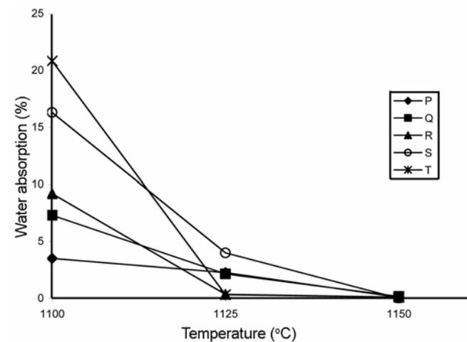
Figure 4. Variation of water absorption against firing temperature.
