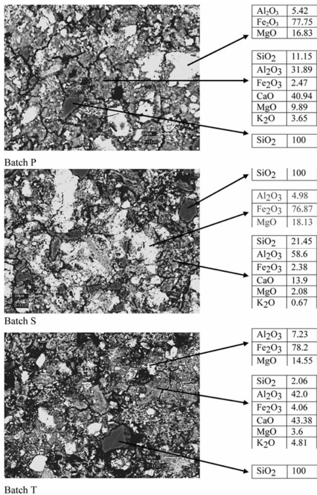
**Figure 7.** Energy dispersive X-ray analysis of the batches fired at 1125°C, represented as the oxide content of the analysed portions.
