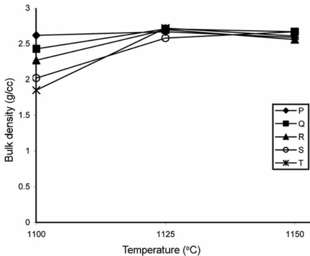
Figure 2. Variation of bulk density against firing temperature.
