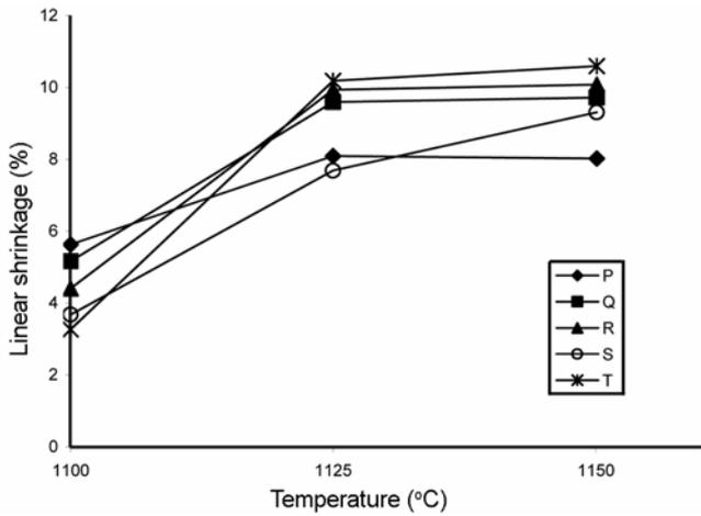
Figure 1. Variation of percent linear shrinkage against firing temperature.
