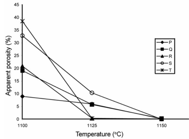
Figure 3. Variation of apparent porosity against firing temperature.
