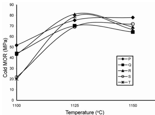
**Figure 5.** Variation of cold strength (MOR) against firing temperature.
