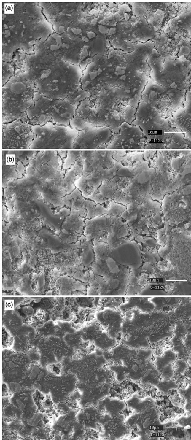
**Figure 6.** Scanning electron micrographs of the (a) batch P, (b) batch A and (c) batch T fired at 1125°C.
