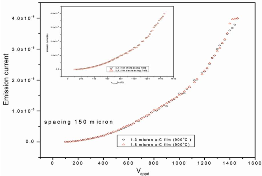
**Figure 9.**  $I$ – $V$  plot of  $a$ -C film of thickness, 1.3  $\mu\text{m}$  and 1.8  $\mu\text{m}$  and the inset is the  $I$ – $V$  plot of increasing and decreasing applied fields.
