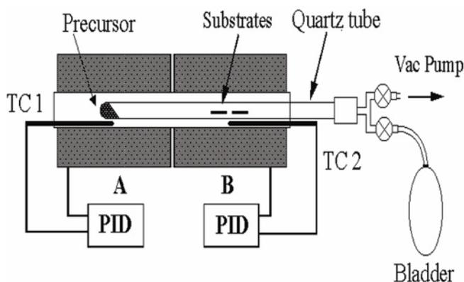
**Figure 1.** Double zone pyrolysis setup.
