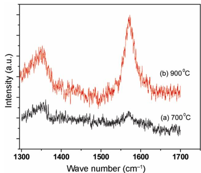
**Figure 4.** Raman spectra of  $a$ -C films prepared at (a) 700°C and (b) 900°C.
