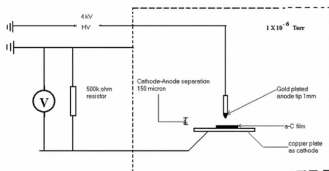
**Figure 7.** Schematic diagram of electron field emission setup.
