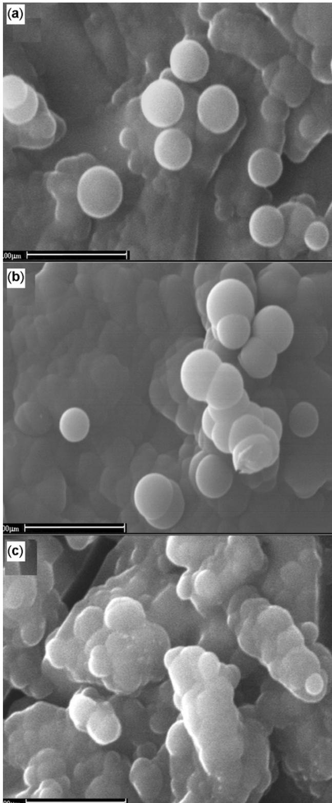
**Figure 3.** SEM images of  $a$ -C films prepared at (a) 700°C, (b) 800°C and (c) 900°C.
