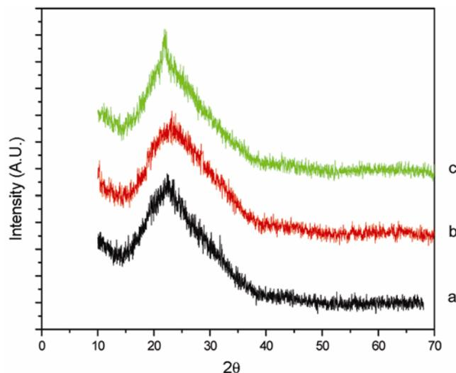
**Figure 2.** XRD pattern of *a*-C films prepared at (a)  $700^\circ\text{C}$ , (b)  $800^\circ\text{C}$  and (c)  $900^\circ\text{C}$ .
