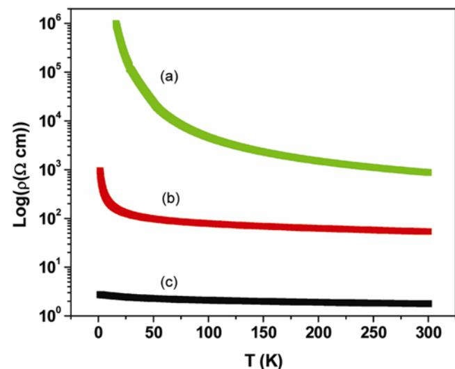
**Figure 5.** (a) Resistivity plot with respect to temperature for the  $a$ -C films prepared at (a) 700°C, (b) 800°C and (c) 900°C.
