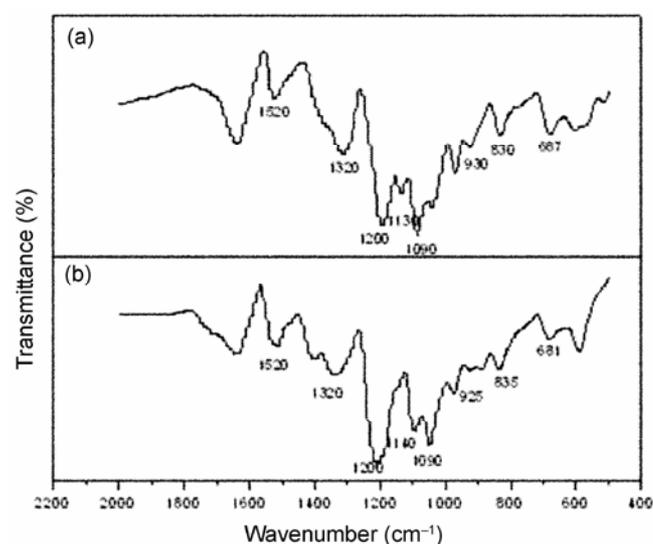
**Figure 1.** FT-IR spectra for (a) PEDOT-PSSA powder and (b) 40 wt.% Pt/PEDOT-PSSA composite.
