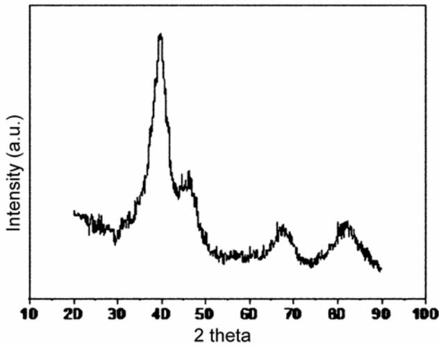
**Figure 2.** Powder X-ray diffraction pattern for Pt/PEDOT-PSSA composite.
