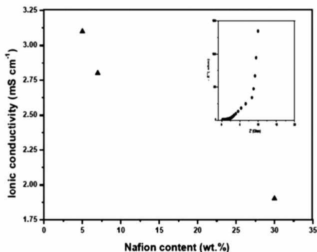
**Figure 7.** Ionic conductivity of electrodes containing 40 wt.% Pt on PEDOT–PSSA with varying Nafion contents. The inset shows the impedance plot of 40 wt.% Pt on PEDOT–PSSA between 65 kHz and 0.1 Hz in aqueous 0.5 M sulphuric acid.
