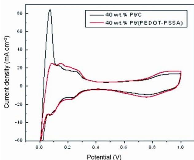
**Figure 5.** CVs for Pt/PEDOT-PSSA and Pt/C in single cell mode with  $\text{H}_2$  and  $\text{N}_2$  streams at anode and cathode, respectively, at room temperature (scan rate =  $50 \text{ mV s}^{-1}$ ).
