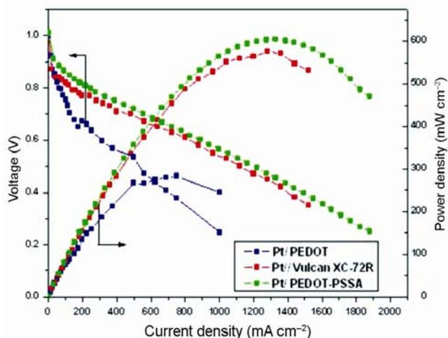
**Figure 9.** Performance curves for PEFCs with 40 wt.% Pt on Vulcan XC-72R, PEDOT and PEDOT-PSSA having 7 wt.% and 30 wt.% Nafion on anodes and cathodes, respectively.
