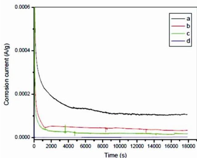
**Figure 6.** Chronoamperometric curves for (a) 40 wt.% Pt/Vulcan XC-72R, (b) 40 wt.% Pt/PEDOT-PSSA composite, (c) Vulcan XC-72R and (d) PEDOT-PSSA composite measured at 0.9 V in  $0.5 \text{ M H}_2\text{SO}_4$ .
