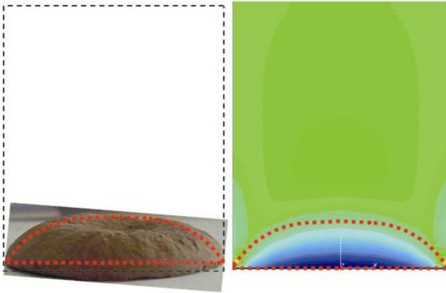
**Figure 5.** Comparison between the cracking cone profile (in red dots) and the stress isovalues after compaction.
