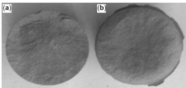
**Figure 2.** Fracture of the compacted powder after ejection.
