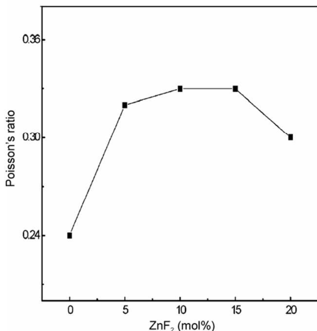
Figure 3. Variation of Poisson's ratio with  $\text{ZnF}_2$  mol%.
