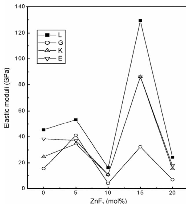
**Figure 2.** Variation of elastic moduli with  $\text{ZnF}_2$  mol%.
