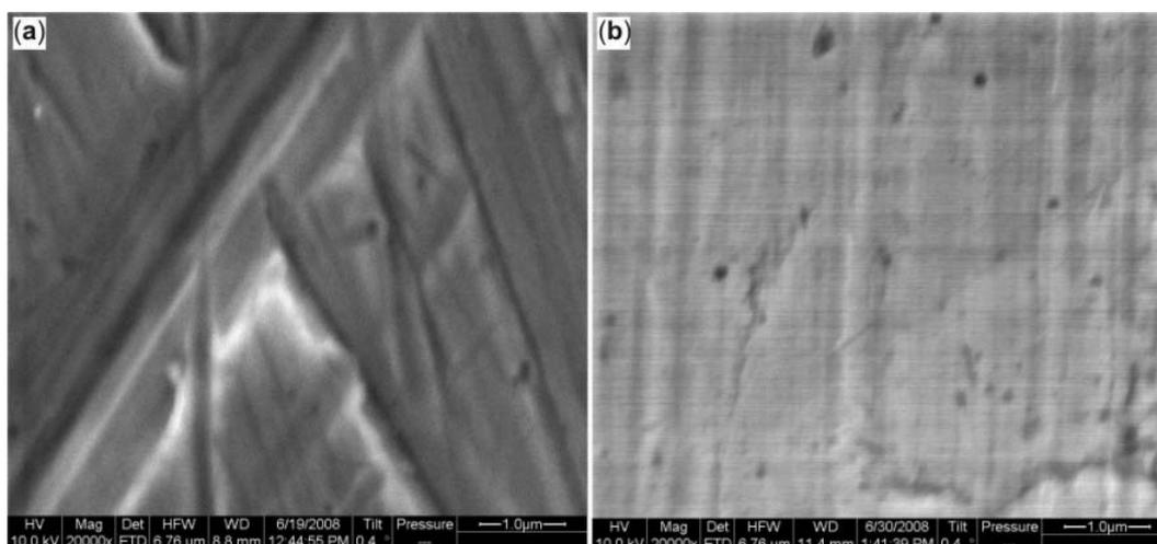
**Figure 2.** Typical SEM images of **a.** DLC film with electron acceleration at 10 kV and a magnification of 20 kX and **b.** bare steel with electron acceleration at 10 kV and a magnification of 20 kX.
