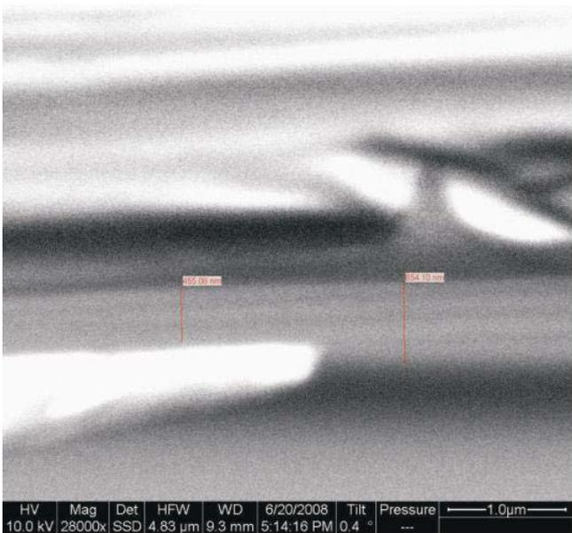
Figure 4. Typical backscattered SEM image of DLC film with electron acceleration at 10 kV and a magnification at 28 kX.
