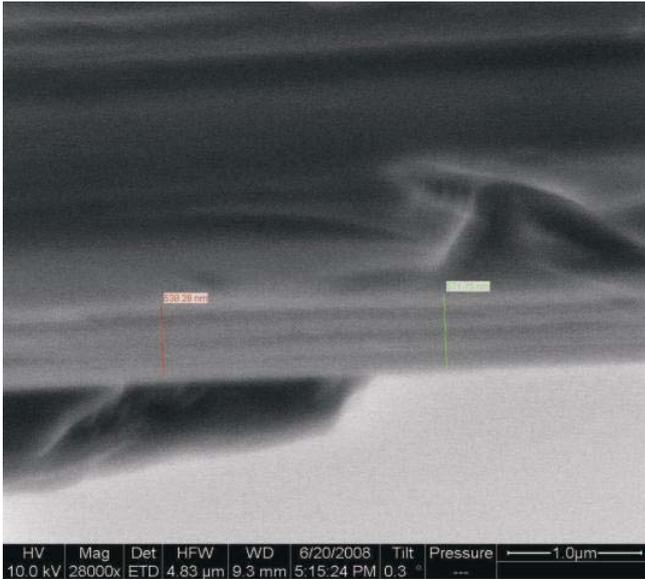
Figure 3. Typical cross-sectional SEM image of DLC film with electron acceleration at 10 kV and a magnification at 28 kX.
