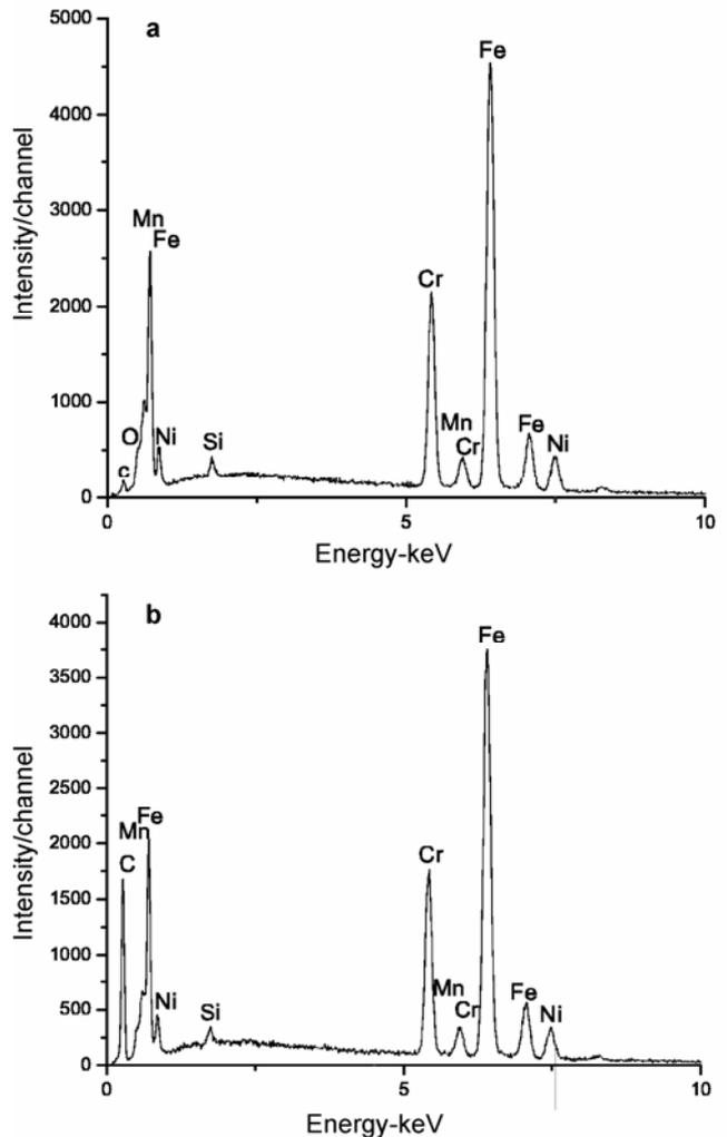
Figure 5. Typical EDX spectra of a. bare steel and b. steel coated with DLC thin film.
