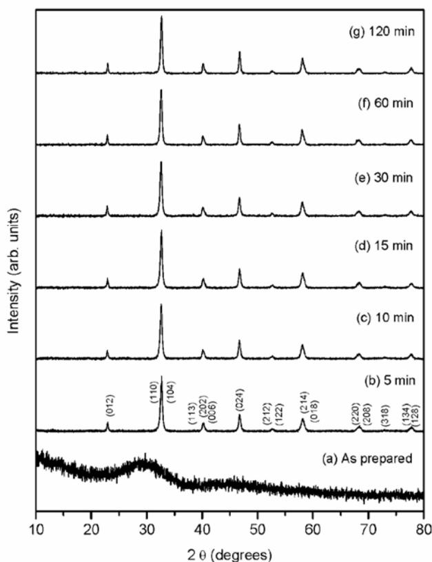
**Figure 1.** Powder X-ray diffraction patterns of  $\text{La}_{0.85}\text{K}_{0.15}\text{MnO}_3$  (a) as prepared and (b–g) calcined at  $800^\circ\text{C}$  from 5 min to 2 h.
