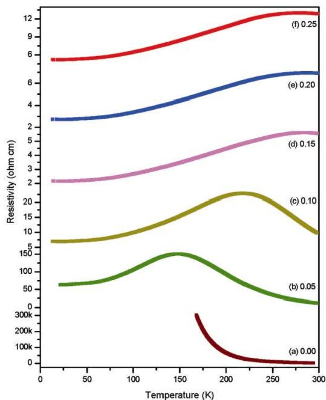
**Figure 6.** Plots of electrical resistivity as a function of temperature for  $\text{La}_{1-x}\text{K}_x\text{MnO}_3$  ( $0.0 \leq x \leq 0.25$ ) compounds, pellets sintered at  $800^\circ\text{C}$  for 12 h.
