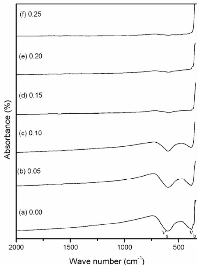
**Figure 5.** FTIR spectra of  $\text{La}_{1-x}\text{K}_x\text{MnO}_3$  ( $0.00 \leq x \leq 0.25$ ) compounds sintered at  $800^\circ\text{C}$  for 12 h.
