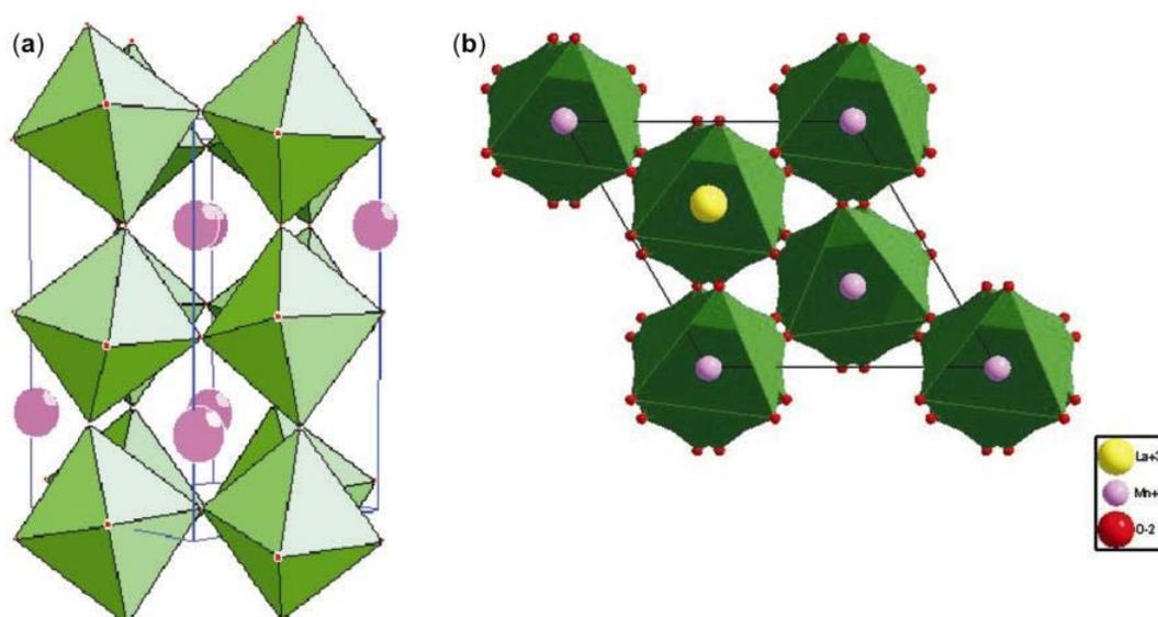
**Figure 4.** Crystal structures of (a) parent  $\text{LaMnO}_3$  in the orthorhombic and (b)  $\text{La}_{0.85}\text{K}_{0.15}\text{MnO}_3$  compound in the rhombohedral structures.
