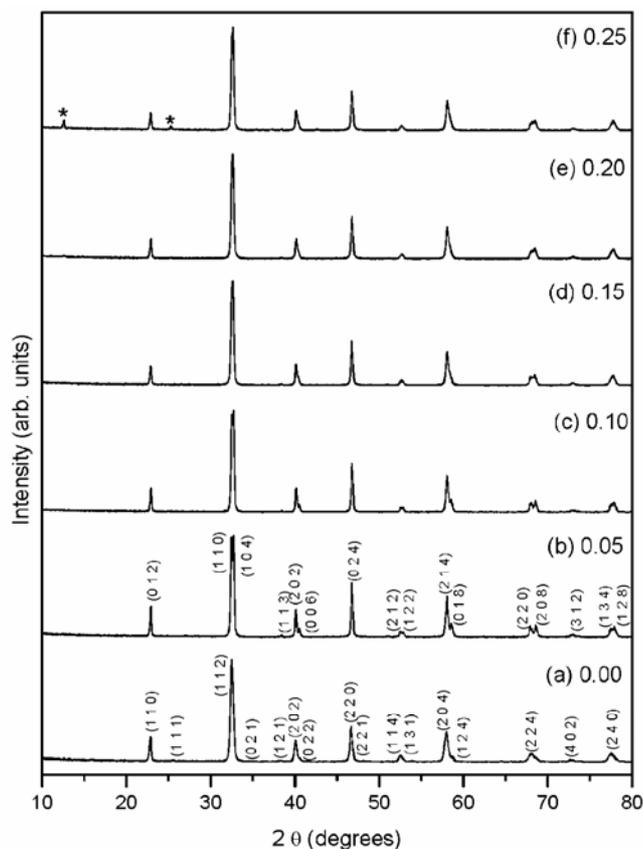
**Figure 2.** Powder X-ray diffraction patterns of  $\text{La}_{1-x}\text{K}_x\text{MnO}_3$  ( $0.00 \leq x \leq 0.25$ ) phases, samples sintered at  $800^\circ\text{C}$  for 12 h (asterisk indicates layered  $\text{K}_x\text{MnO}_2$  impurity phase).
