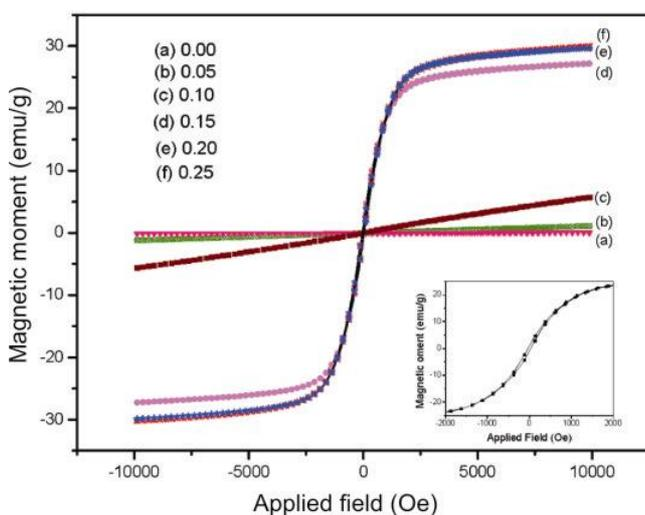
**Figure 9.** Plots of magnetic moment as a function of applied field for  $\text{La}_{1-x}\text{K}_x\text{MnO}_3$  ( $0.00 \leq x \leq 0.25$ ) compounds sintered at  $800^\circ\text{C}$  for 12 h. In the inset, typical hysteresis loop of  $\text{La}_{0.85}\text{K}_{0.15}\text{MnO}_3$  compound is shown.
