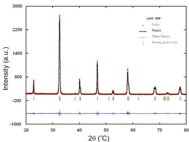
**Figure 3.** Typical observed, calculated and the difference Rietveld refined X-ray diffraction patterns of  $\text{La}_{0.85}\text{K}_{0.15}\text{MnO}_3$  compound.
