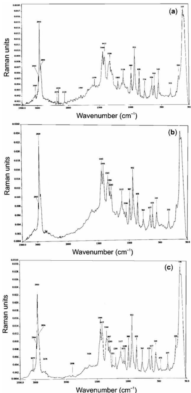
**Figure 3.** FT-Raman spectra of (a) pure LAA, (b) Cu<sup>2+</sup> doped LAA and (c) Mg<sup>2+</sup> doped LAA.
