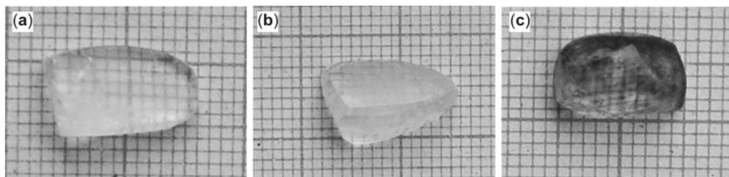
**Figure 1.** Photographs of as grown (a) pure LAA, (b)  $\text{Cu}^{2+}$  doped LAA and (c)  $\text{Mg}^{2+}$  doped LAA crystals.
