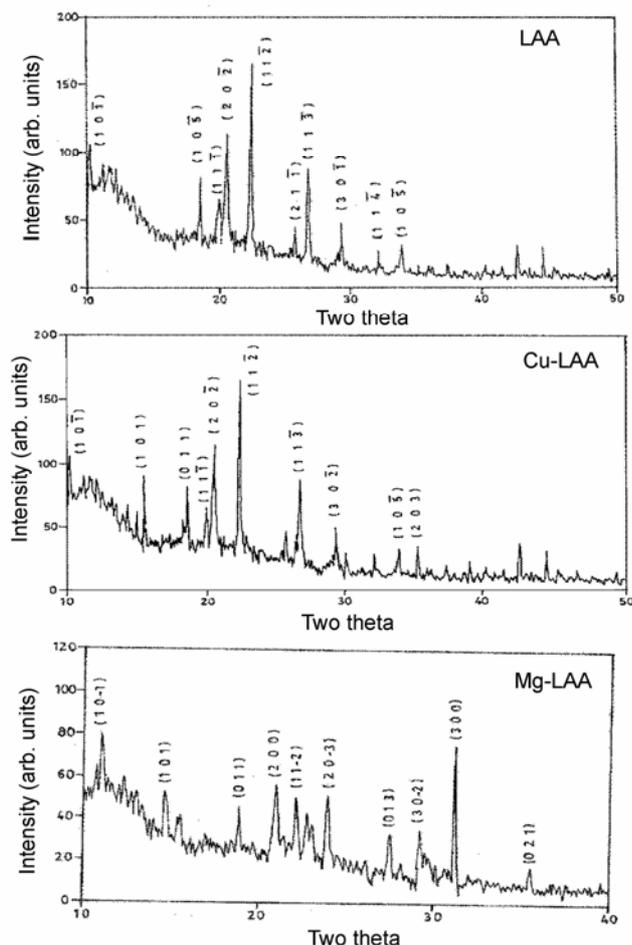
**Figure 2.** Powder X-ray diffraction pattern of LAA, Cu-LAA and Mg-LAA.
