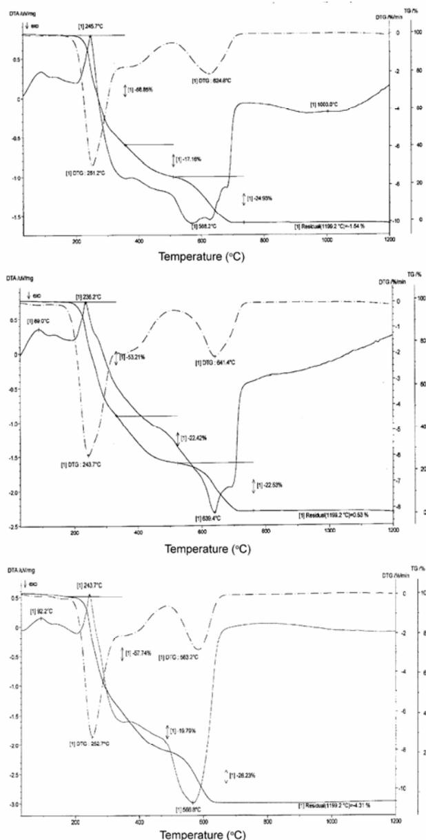
**Figure 5.** TGA, DTA and DTG curves of pure,  $Cu^{2+}$  and  $Mg^{2+}$  doped LAA single crystals.
