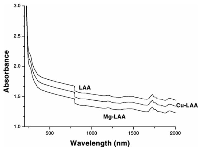
**Figure 4.** Optical absorption spectra of pure, Cu<sup>2+</sup> and Mg<sup>2+</sup> doped LAA.
