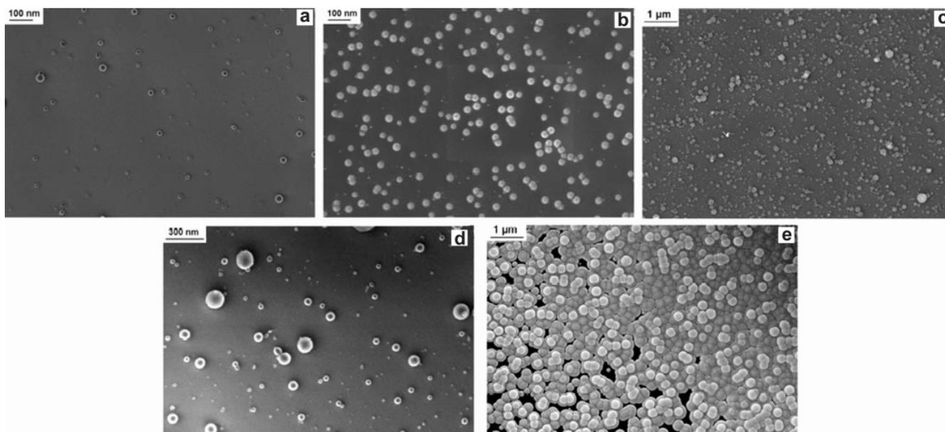
**Figure 6.** SEM images showing the effect of volumetric flow rate on the size and morphology of carbon nanospheres: flow rate **a.** 0.2 ml/h, **b.** 0.8 ml/h, **c.** 1.4 ml/h, **d.** magnified view of **c**; **e.** 2.0 ml/h. Other parameters are electric potential, 2.0 kV/cm and flow rate, 0.8 ml/h.
