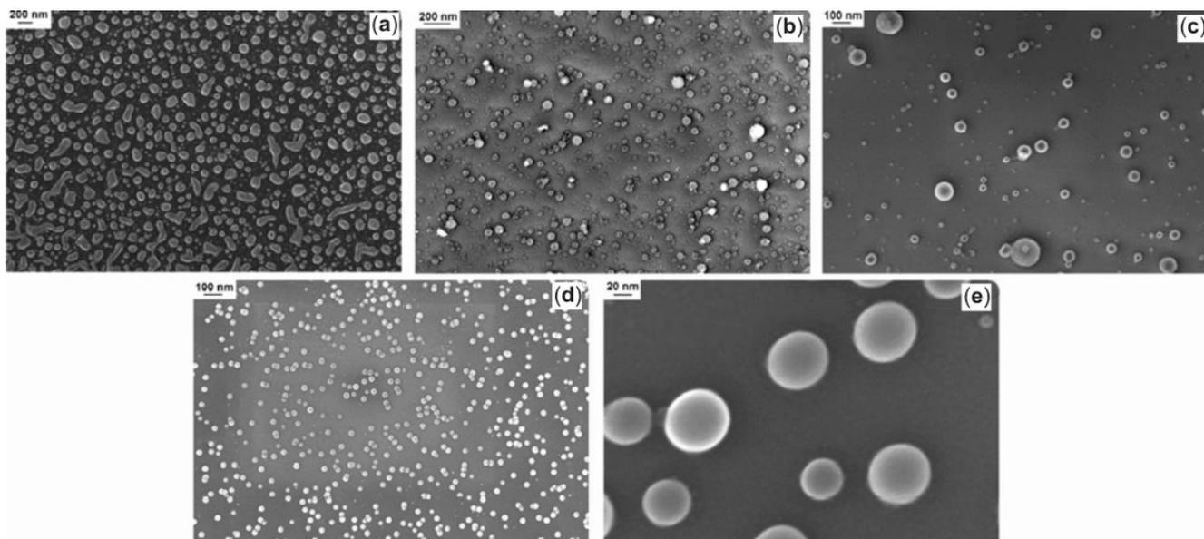
**Figure 4.** SEM images showing the effect of needle gauge on the size and morphology of carbon nanospheres: needle gauge (a) 18 g; (b) 22 g; (c) magnified view of (b); (d) 26 g; (e) magnified view of (d). Other parameters are electric potential, 2.0 kV/cm and flow rate, 0.8 ml/h.
