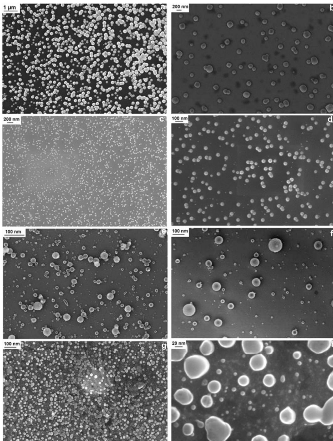
**Figure 5.** SEM images showing the effect of applied electric potential on the size and morphology of carbon nanospheres: electric potential. **a.** 1.0 kV/cm; **c.** 1.5 kV/cm; **e.** 2.0 kV/cm; **g.** 2.5 kV/cm. Images **b, d, f** and **h** are magnified view of **a, c, e** and **g**, respectively. Other parameters are needle gauge, 26 and flow rate, 0.8 ml/h.
