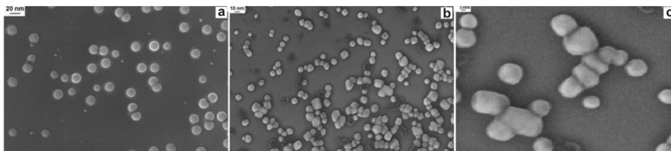
**Figure 7.** SEM images of carbon nanospheres at optimized parameters (needle gauge 26 g, applied electric potential: 1.5 kV/cm and flow rate: 0.8 ml/h) derived by two different types of RF sol: **a.** acetone based, **b.** water based, and **c.** magnified view of **b**. Scale bars correspond to 20, 10 and 5 nm, respectively in **a–c**.
