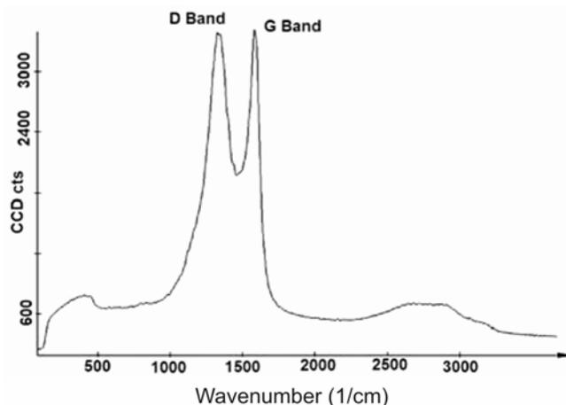
Figure 2. Raman spectrum of RF derived carbon nanospheres.
