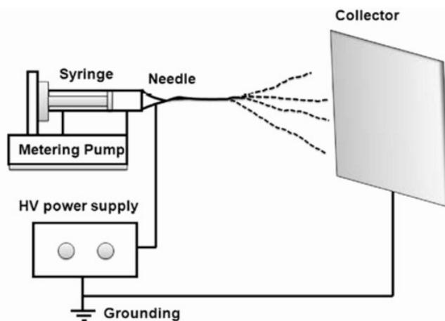
Figure 1. Schematic diagram of electro spraying set-up.
