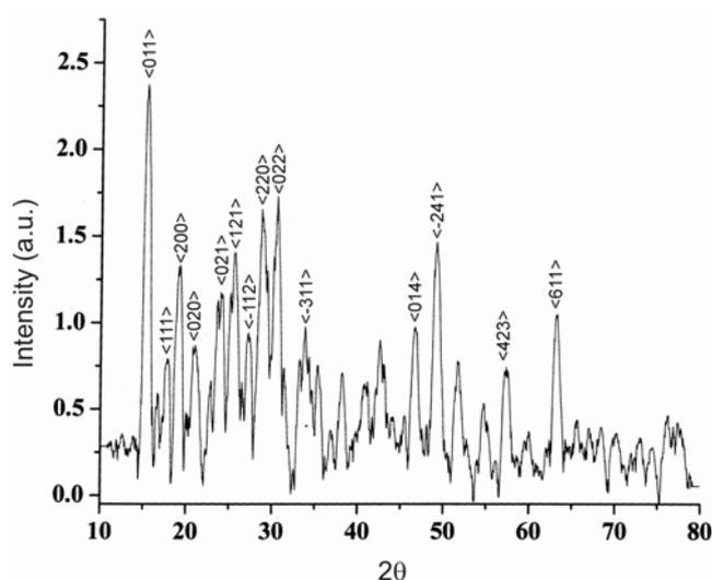
**Figure 3.** X-ray diffractogram of barium calcium iodate.
