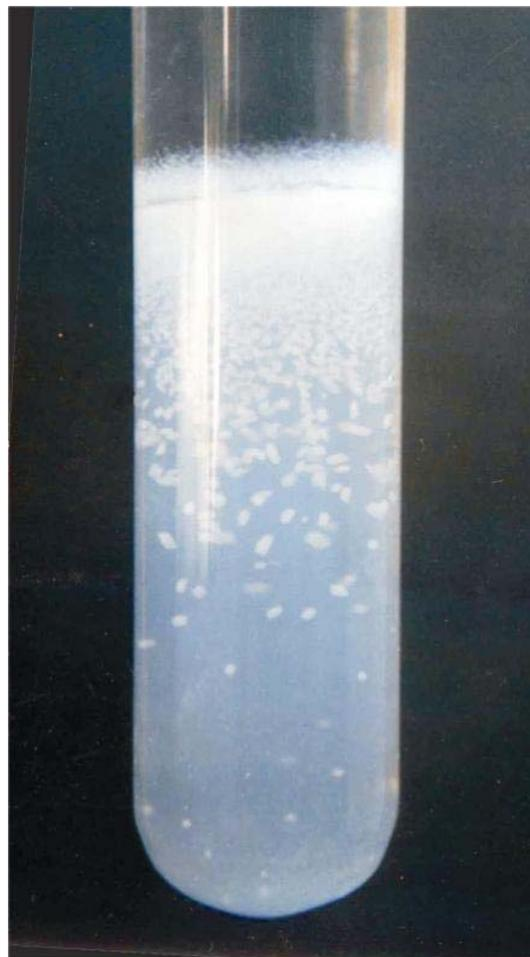
**Figure 1.** Dendritic growth of barium-calcium iodate crystals.
