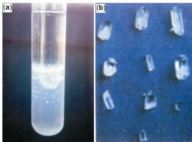
**Figure 2.** (a) Prismatic transparent crystals of barium calcium iodate inside the test tube and (b) few prismatic transparent crystals of barium calcium iodate.
