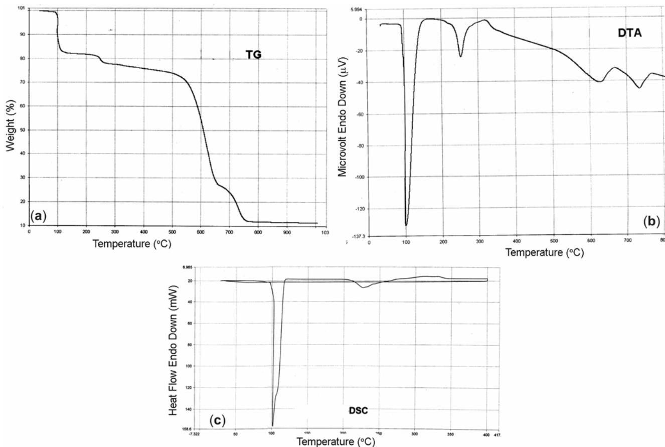
**Figure 5.** (a) TGA curve of barium calcium iodate crystal, (b) DTA curve of barium calcium iodate crystal and (c) DSC curve of barium calcium iodate crystal.
