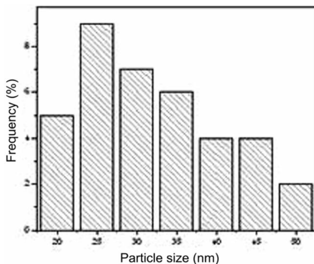
Figure 4. Particle distribution obtained from TEM image.
