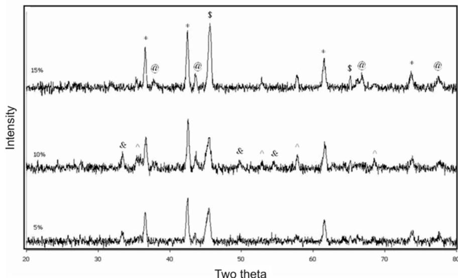
**Figure 5.** X-ray diffraction patterns of the FeTiO<sub>3</sub>–C–Al ternary system that was heated in microwave furnace for 20 min with 5, 10 and 15%wt Al (TiC (\*), Fe (\$), SiC (@), Al<sub>2</sub>O<sub>3</sub> (^), Fe<sub>2</sub>O<sub>3</sub> (&)).
