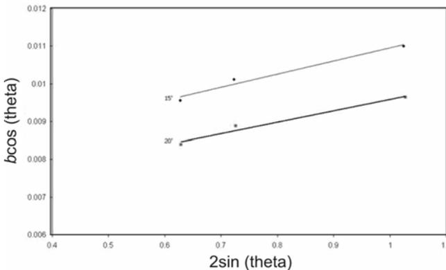
**Figure 3.** Williamson–Hall diagram of the  $\text{FeTiO}_3$ –C system for specimens heated in microwave for 15 and 20 min.
