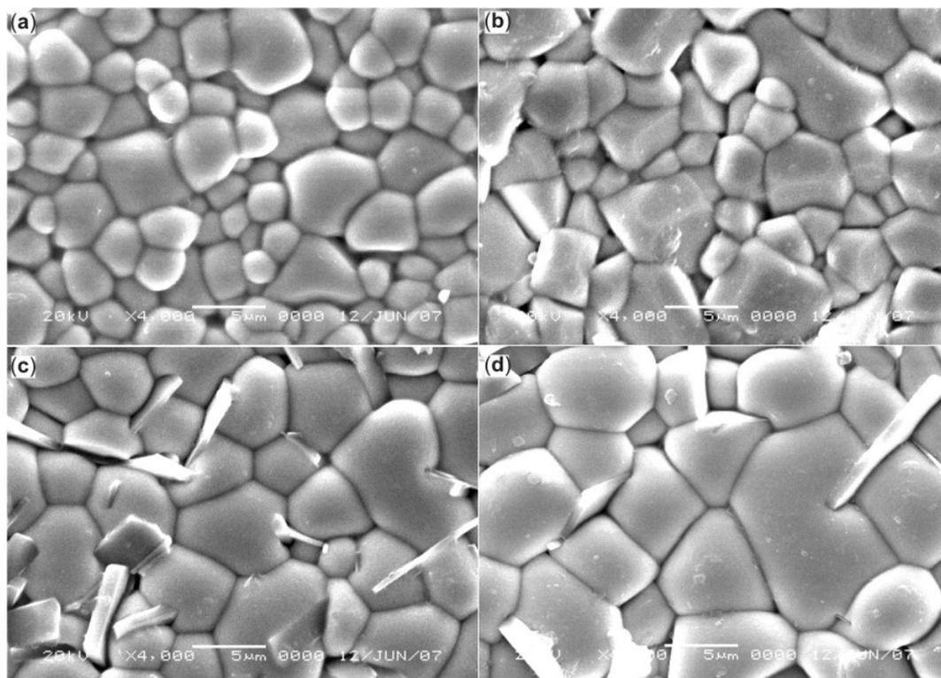
**Figure 2.** SEM micrographs of  $(\text{Bi}_{1/2}\text{Na}_{1/2})\text{Ti}_{1-x}(\text{Mg}_{1/3}\text{Nb}_{2/3})_x\text{O}_3$  ceramics with (a)  $x = 0.005$ , (b)  $x = 0.010$ , (c)  $x = 0.015$  and (d)  $x = 0.020$ .
