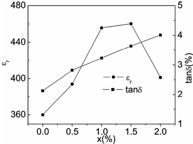
**Figure 4.** Dielectric constant,  $\epsilon_r$  and dielectric loss  $\tan\delta$  of  $(\text{Bi}_{1/2}\text{Na}_{1/2})\text{Ti}_{1-x}(\text{Mg}_{1/3}\text{Nb}_{2/3})_x\text{O}_3$  ceramics as a function of  $x$ .
