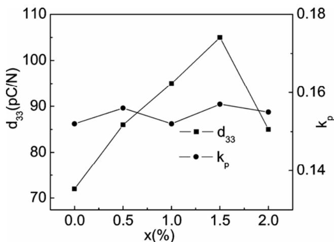
**Figure 3.** Piezoelectric constant,  $d_{33}$  and planar electro-mechanical coupling factor,  $k_p$ , of  $(\text{Bi}_{1/2}\text{Na}_{1/2})\text{Ti}_{1-x}(\text{Mg}_{1/3}\text{Nb}_{2/3})_x\text{O}_3$  ceramics as a function of  $x$ .
