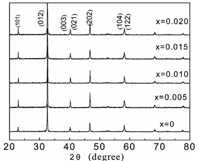
Figure 1. XRD patterns of  $(\text{Bi}_{1/2}\text{Na}_{1/2})\text{Ti}_{1-x}(\text{Mg}_{1/3}\text{Nb}_{2/3})_x\text{O}_3$  ceramics.
