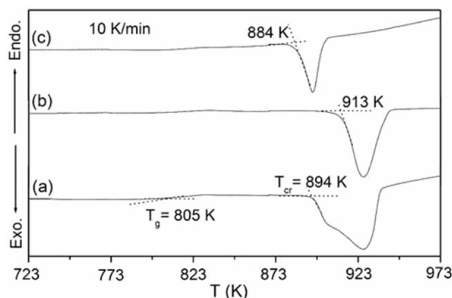
Figure 2. DSC traces for (a) seeded  $\text{BaNaB}_9\text{O}_{15}$  glass plate, (b) unseeded  $\text{BaNaB}_9\text{O}_{15}$  glass plate and (c) powder.
