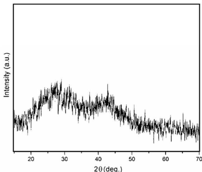
Figure 1. XRD pattern for the as-quenched pulverized  $\text{BaNaB}_9\text{O}_{15}$  glass.
