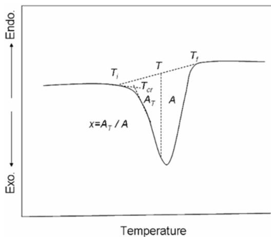
**Figure 4.** Typical exothermic peak in non-isothermal experiment.
