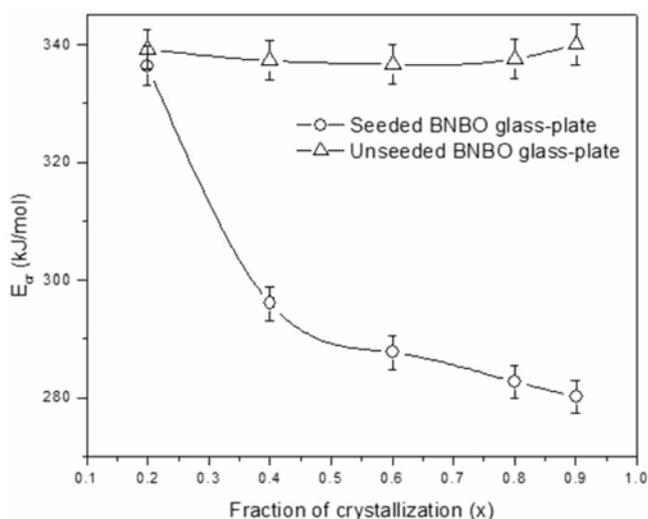
**Figure 7.** Variation of activation energy with the fraction of crystallization for both the seeded and unseeded glasses.
