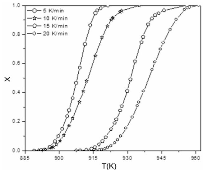
**Figure 5.** Fraction of crystallization vs temperature curves at various heating rates for seeded BNBO glass plates.
