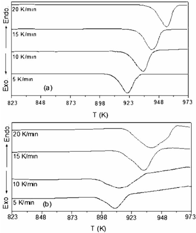
**Figure 3.** DSC traces for the (a) as-quenched unseeded and (b) seeded BaNaB<sub>9</sub>O<sub>15</sub> glass plates at different heating rates.
