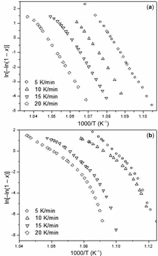
**Figure 6.**  $\ln[-\ln(1-x)]$  vs  $1000/T$  plots for (a) unseeded and (b) seeded BNBO glass plates at various heating rates.
