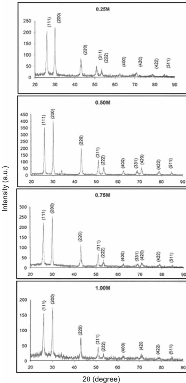
**Figure 1.** X-ray diffraction patterns of PbS films for different molarities.
