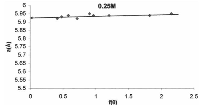
**Figure 2.** Nelson–Riley plot for a PbS thin film.
