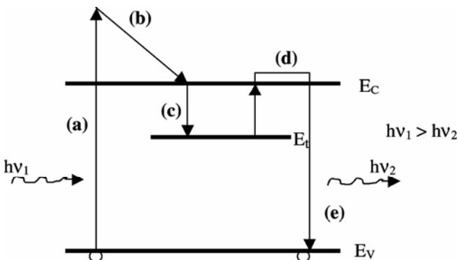
**Figure 4.** Direct excitation and recombination mechanisms in semiconductor with a trapping level for electrons.
