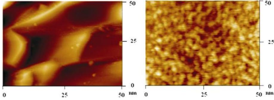
**Figure 6.** AFM micrograph of samples A and B etched at laser power,  $30 \text{ W/cm}^2$ , for etching time, 45 min.
