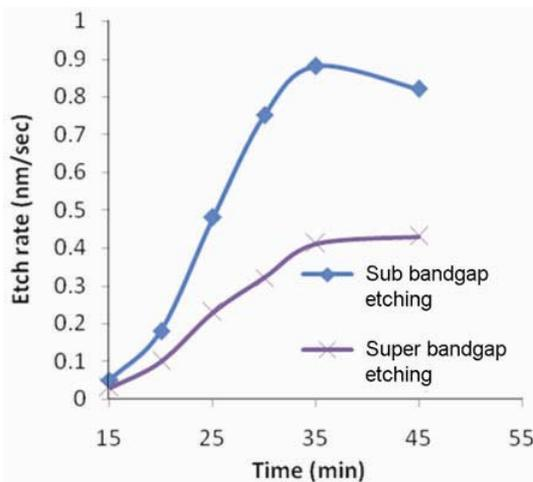
**Figure 2.** The etching rate as a function of etching duration for sample A.
