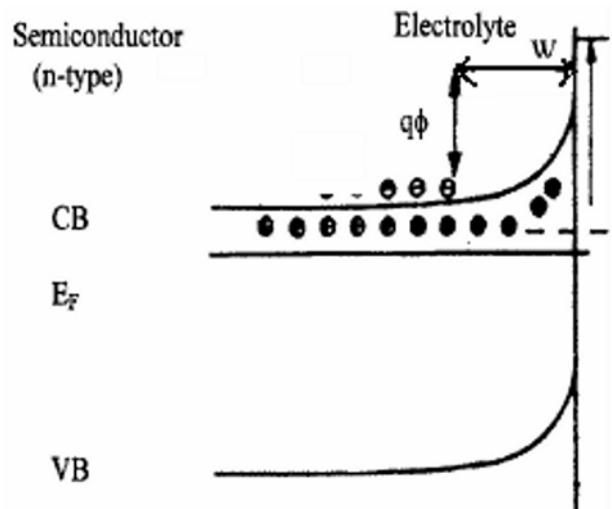
**Figure 3.** Schematic illustration of the band model for n-type semiconductor/electrolyte junction under photon illumination.
