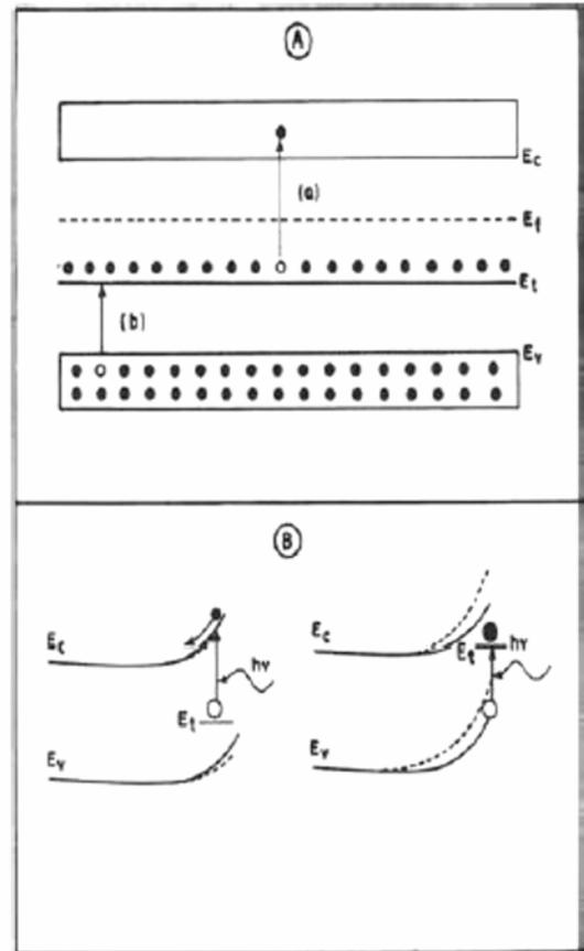
**Figure 5.** Schematic band diagrams of the surface space charge region at semiconductor/electrolyte interface under sub-bandgap illumination with excitation of trapped (A) electrons and (B) holes.  $E_t$  represents one defect state below  $E_f$  at equilibrium.
