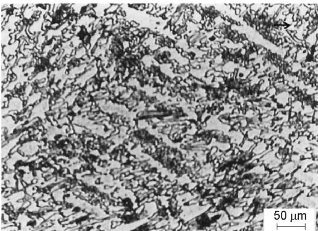
**Figure 6.** Optical photomicrograph of AC sand mould 10% manganese bearing sample (200X).
