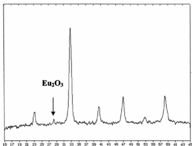
**Figure 3.** X-ray diffraction pattern of  $\text{La}_{1-x}\text{Eu}_x\text{Mn}_{0.9}\text{Zn}_{0.1}\text{O}_{3+d}$  for  $x = 0.4$ .
