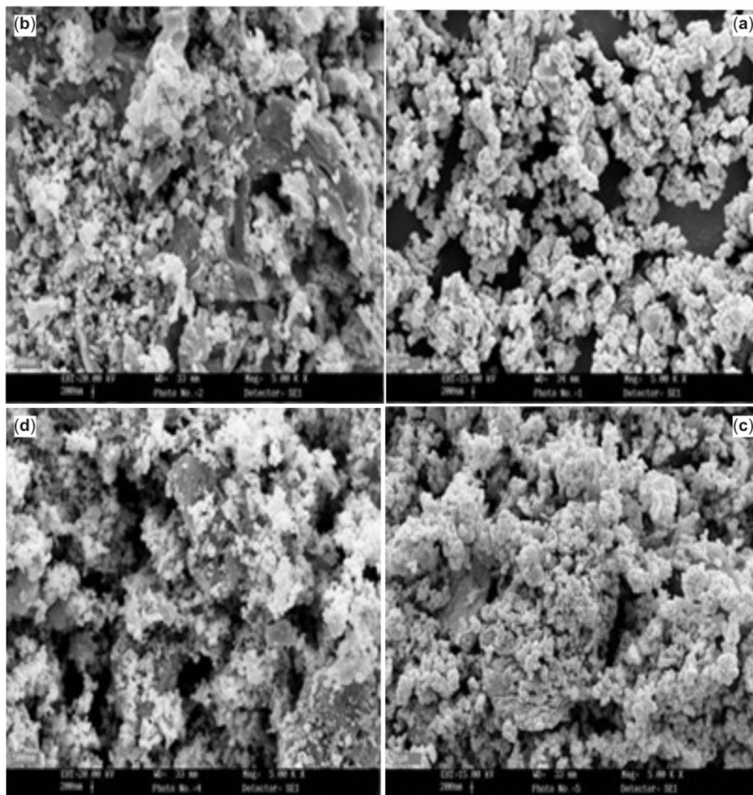
**Figure 5.** SEM images of (a)  $\text{LaMn}_{0.9}\text{Zn}_{0.1}\text{O}_{3+d}$ , (b)  $\text{La}_{0.9}\text{Eu}_{0.1}\text{Mn}_{0.9}\text{Zn}_{0.1}\text{O}_{3+d}$ , (c)  $\text{La}_{0.8}\text{Eu}_{0.2}\text{Mn}_{0.9}\text{Zn}_{0.1}\text{O}_{3+d}$  and (d)  $\text{La}_{0.68}\text{Eu}_{0.32}\text{Mn}_{0.9}\text{Zn}_{0.1}\text{O}_{3+d}$  calcined at  $800^\circ\text{C}$  in air.
