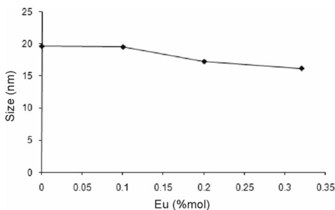
**Figure 6.** Particle sizes of  $\text{La}_{1-x}\text{Eu}_x\text{Mn}_{0.9}\text{Zn}_{0.1}\text{O}_{3+d}$  calcined at  $800^\circ\text{C}$  versus molar ratio of  $\text{Eu}^{3+}$ . Average particle diameter decreases with increasing europium content.
