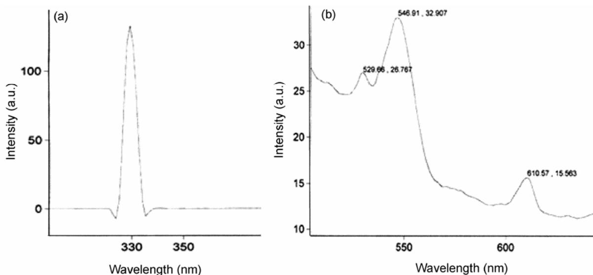
**Figure 8.** Excitation (a) ( $\lambda = 330$  nm) and emission (b) ( $\lambda = 547$  nm) spectra of  $\text{La}_{0.68}\text{Eu}_{0.32}\text{Mn}_{0.9}\text{Zn}_{0.1}\text{O}_{3+d}$  nano powders annealed at  $800^\circ\text{C}$ .
