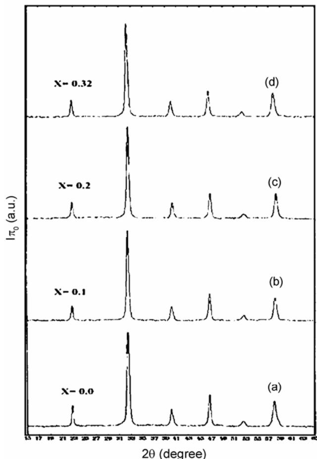
**Figure 2.** X-ray diffractogram of  $\text{La}_{1-x}\text{Eu}_x\text{Mn}_{0.9}\text{Zn}_{0.1}\text{O}_{3+d}$  calcined at  $800^\circ\text{C}$ : (a)  $x = 0.0$ ; (b)  $x = 0.1$ ; (c)  $x = 0.2$  and (d)  $x = 0.32$ .
