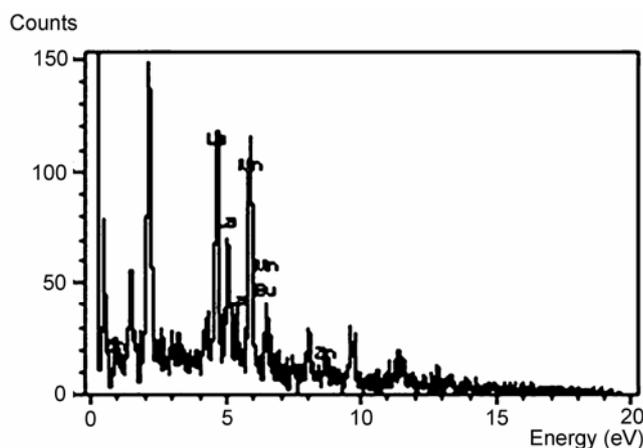
**Figure 7.** Energy dispersive spectra (EDX) of  $\text{La}_{0.68}\text{Eu}_{0.32}\text{Mn}_{0.9}\text{Zn}_{0.1}\text{O}_{3+d}$ .
