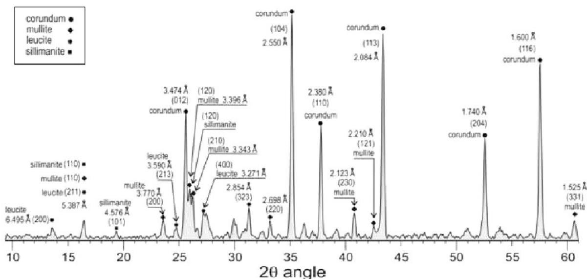
**Figure 2.** X-ray diffractogram performed on a white opaque grain. It is possible to distinguish 43% of corundum ( $\text{Al}_2\text{O}_3$ ), 22% of mullite [72% of  $\text{Al}_2\text{O}_3$  and 28% of  $\text{SiO}_2$ ], 12% of leucite ( $\text{KAlSi}_2\text{O}_6$ ) and 23% of sillimanite [ $\text{Al}_2\text{O}_3 \cdot \text{SiO}_2$ ].
