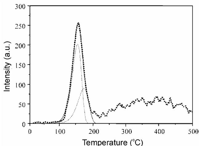
**Figure 4.** Natural TL glow curve of alumina removed from the refractory brick. The well-defined peak at lower temperature can be deconvoluted into two components (peaked at 157 and 177°C) assuming first order kinetics.
