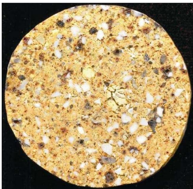
**Figure 1.** Slice of one of the twenty analysed refractory bricks cut using a water-lubricated diamond blade.
