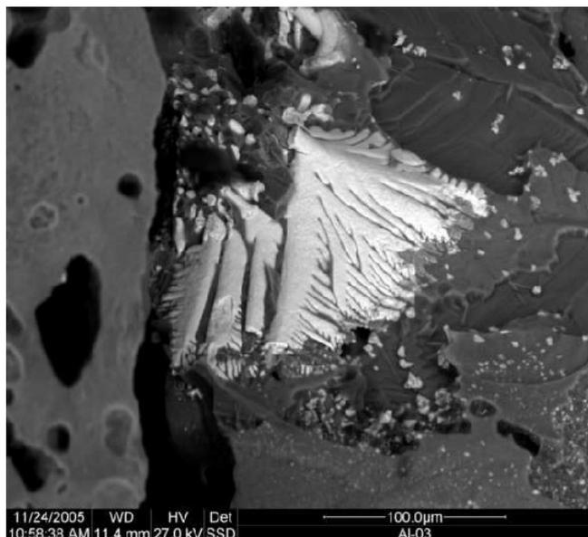
**Figure 3.** Detail of a SEM picture where  $\text{ZrO}_2$  is observed on the surface of some alumina grains.
