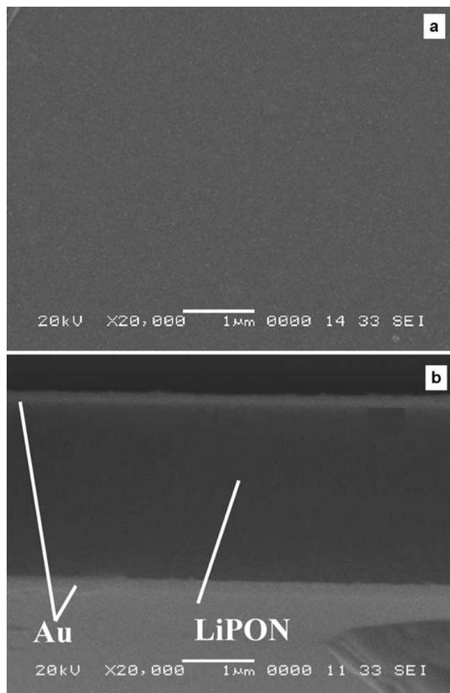
**Figure 2.** SEM images of a. surface of LiPON on Au film and b. cross-section of Au/LiPON/Au sandwich structure. (Deposition conditions: rf power is  $5.5 \text{ W/cm}^2$ , and nitrogen gas pressure is  $1.5 \text{ Pa}$ ).
