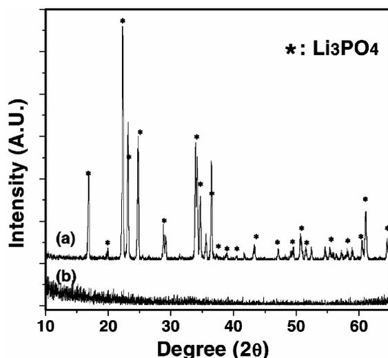
**Figure 1.** Typical X-ray diffraction patterns of (a)  $\text{Li}_3\text{PO}_4$  target and (b) LiPON thin film.
