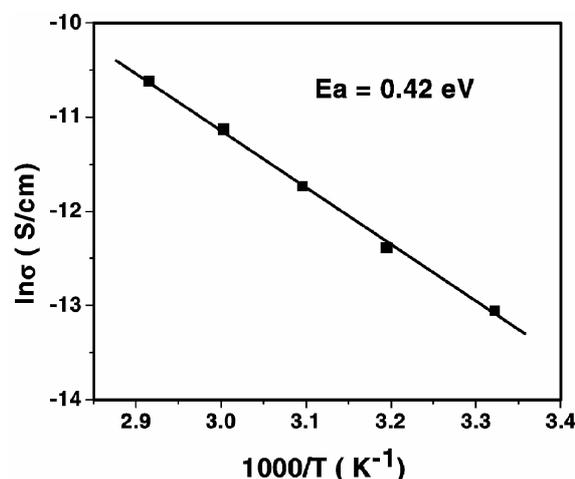
Figure 5. Typical Arrhenius behaviour of ionic conductivity vs temperature. (Deposition conditions: rf power is 5.5 W/cm<sup>2</sup>, and nitrogen gas pressure is 1.5 Pa).
