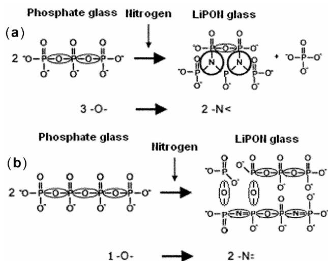
**Figure 9.** Partial structure of nitrided Li<sub>3</sub>PO<sub>4</sub> glass with the incorporation of (a)  $>N<$  and (b)  $=N=$  resulting from the reaction of two adjacent phosphate chains with nitrogen.
