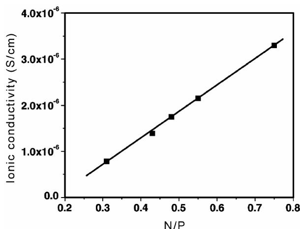
Figure 7. Ionic conductivity of LiPON thin films as a function of N/P ratio.
