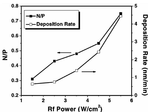
Figure 3. N/P ratio and deposition rate of LiPON thin films as a function of rf power.
