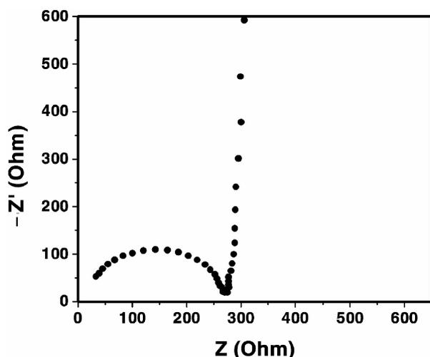
Figure 4. A Nyquist a.c. impedance plot of a LiPON thin film at room temperature. (Deposition conditions: rf power is 5.5 W/cm<sup>2</sup>, and nitrogen gas pressure is 1.5 Pa).
