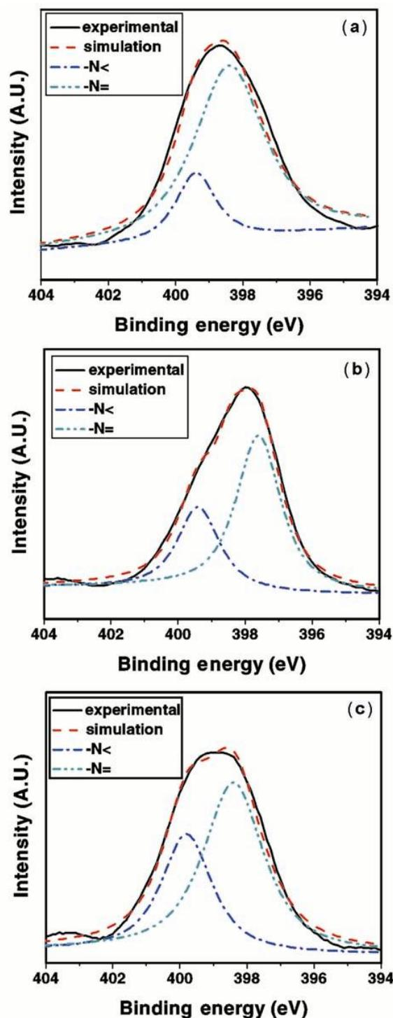
Figure 8.  $\text{N}_{1s}$  XPS spectrum of LiPON thin films deposited at (a)  $1.5 \text{ W/cm}^2$ , (b)  $3.5 \text{ W/cm}^2$ , and (c)  $5.5 \text{ W/cm}^2$ .
