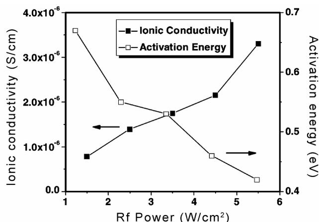
Figure 6. Ionic conductivity and activation energy of LiPON thin films as a function of rf power.
