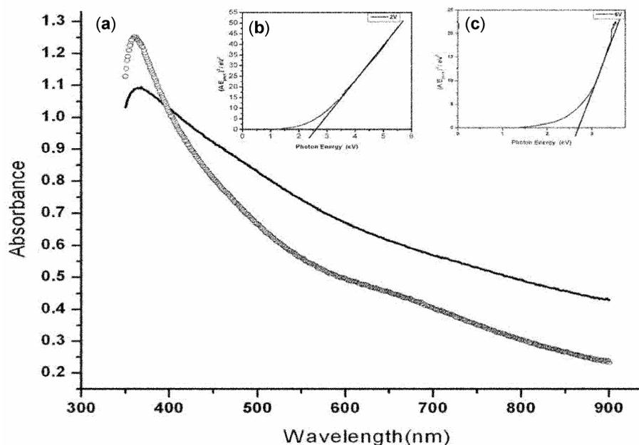
**Figure 3.** (a) UV-visible absorption spectrum of the nanothreads and nanowires like structures synthesized at 2 V and 6 V, (b) and (c) bandgap calculation of the nanothreads and nanowires like structures from the UV-visible absorption spectrum.
