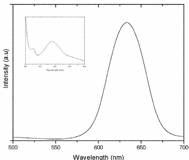
**Figure 6.** Room temperature photoluminescence (PL) spectra of the aligned ZnO nanorods.
