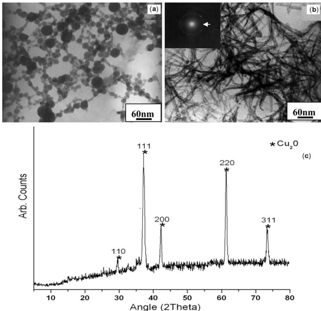
**Figure 1.** (a) Typical transmission electron micrograph of Cu<sub>2</sub>O nanothreads embodying beads, as collected at the bottom of the cell after electrolysis at 2 V for 1 h, (b) is the representative TEM micrograph of dense Cu<sub>2</sub>O network of nanowires, obtained after electrolysis at 6 and 10 V, respectively for 1 h and (c) is the X-ray diffraction of the as obtained materials at the bottom of the electrolytic cell after electrolysis at 6 V.
