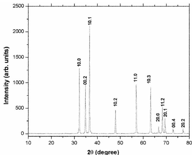
**Figure 5.** XRD pattern of as-grown ZnO sample.
