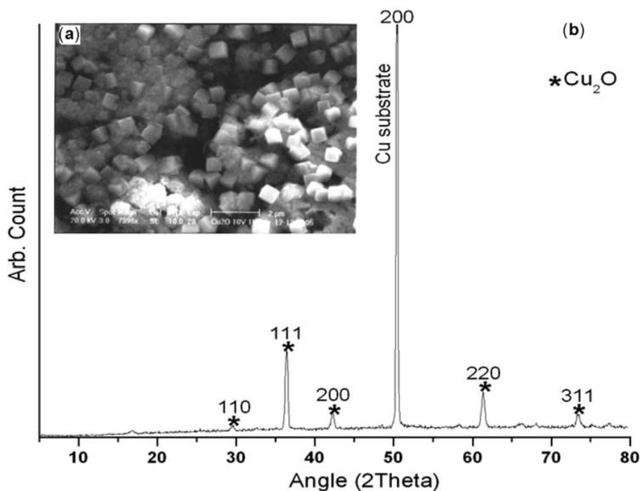
**Figure 2.** (a) SEM micrographs of the copper electrode after electrolysis at 10 V and (b) XRD pattern of the copper sheet after electrolysis at 10 V for 1 h.
