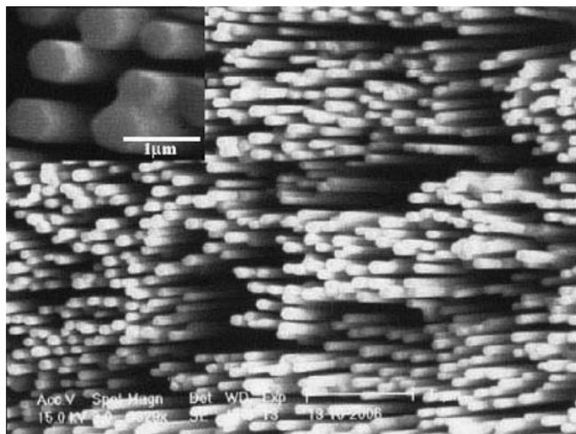
**Figure 4.** A low magnification SEM image of the aligned ZnO nanorods. The inset is the high magnification SEM image.
