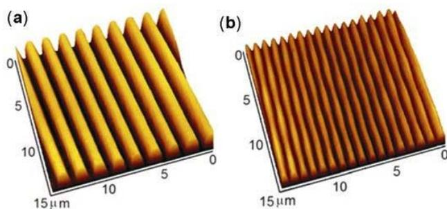
**Figure 1.** AFM scans of the peeled patterned foils of (a) a compact disc (CD) (stripe periodicity,  $1.5 \mu\text{m}$ ; stripe width,  $750$  nm; stripe height,  $130$  nm) and (b) a DVD (stripe periodicity,  $800$  nm, stripe width,  $\sim 400$  nm; stripe height,  $\sim 70$  nm).
