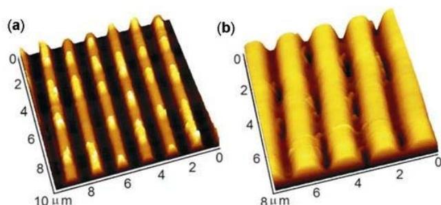
**Figure 10.** (a) AFM image of a patterned foil of a data containing CD with an array of raised pillars along the tracks and (b) a  $850 \text{ nm}$  thick PDMS film, imprinted with a data containing CD foil, resulting in structures having array of pits along the channels.
