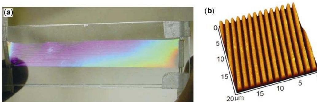
**Figure 2.** (a) Digicam image of a  $10 \times 40$  mm patterned flexible PVA foil and (b) AFM scan of the foil shown in (a), showing that the stripe periodicity is  $1.5 \mu\text{m}$ , stripe width,  $750 \text{ nm}$  and stripe height,  $130 \text{ nm}$ .
