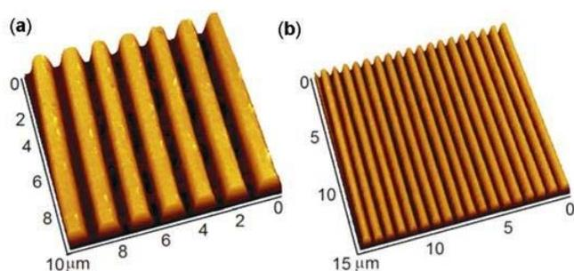
**Figure 7.** AFM images of negative replicas of foil patterns on hydrogel (PAA) films obtained by adhesion assisted imprint lithography. (a) Stamp used is a CD foil and (b) a DVD foil. The film thickness were  $3.5$   $\mu\text{m}$  and  $6.1$   $\mu\text{m}$ , respectively.
