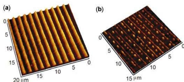
**Figure 8.** AFM images of patterns obtained on thin PMMA films coated on flat silicon wafer substrate by solvent vapour assisted imprinting at room temperature using flexible patterned PVA foils. (a) A 168 nm thick PMMA film imprinted to form a perfect negative replica of the stamp and (b) imprinting of a 59 nm thick PMMA film under a patterned PVA stamp resulted in confined dewetting of the film, with formation of aligned dewetted structures.
