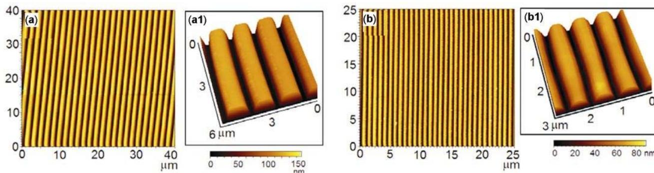
**Figure 4.** Typical AFM images of negative replicas of foil patterns on cross-linked PDMS films. Stripe patterns obtained using (a) a CD foil (film thickness, 3.1 μm), and (b) a DVD foil (film thickness, 2.2 μm). Heights of the polymer patterns match with the height of foil patterns. Insets are 3-D AFM images, which clearly show the high fidelity of the patterns in case of using CD foils and arch like cross-section while using DVD foils.
