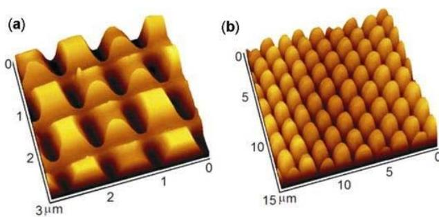
**Figure 5.** AFM images of two-dimensional cross patterns obtained by multiple imprinting. (a) 350 × 350 nm, pillars obtained by multiple imprinting using a DVD stamp. The second imprint was at right angles to the direction of the first imprint and the film thickness was ~2.3 μm and (b) rhombic columns obtained by imprinting the PDMS film twice with a CD stamp, by making the second imprint at an angle of 45° relative to the first. The film thickness was ~1.9 μm.
