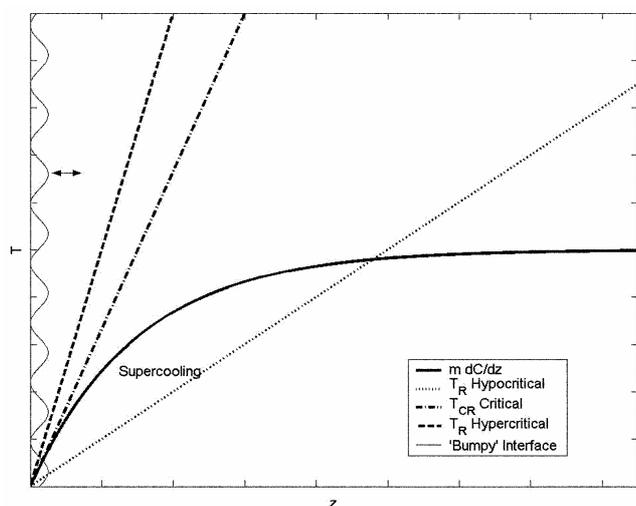
**Figure 2.** Condition for shape instability and stability as per constitutional supercooling.
