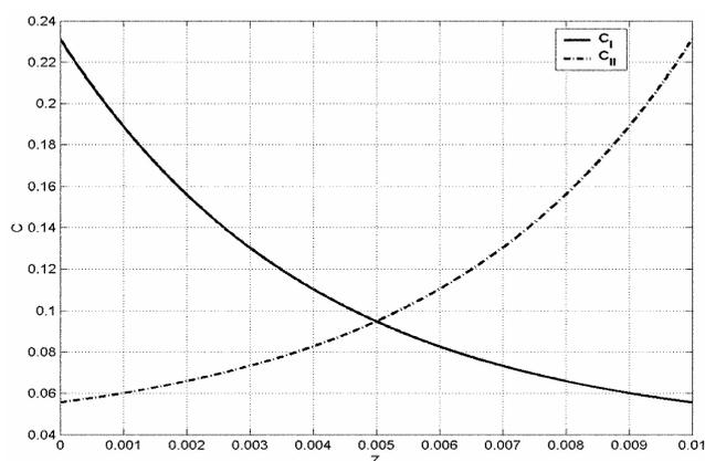
**Figure 3.** Diffusion fields of converging interfaces, Al-4Cu system,  $\Delta = 0.01$  cm.
